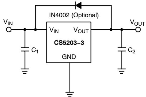
Figure 9. Protection Diode Scheme for Large Output Capacitors
