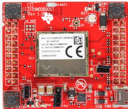
**Figure 1. CC3100MOD BoosterPack Board With the CC3100MOD**
