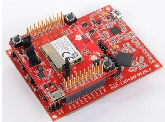
Figure 16. CC3100MODBOOST Connected to MSP430F5529 LaunchPad
