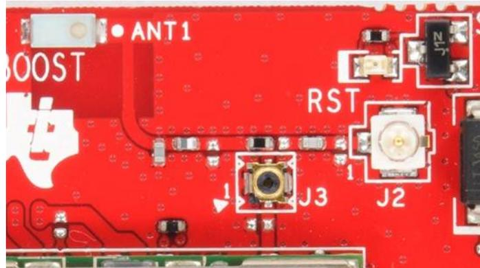
Figure 12. Resistor Switch for Radiated versus Conducted Tests
