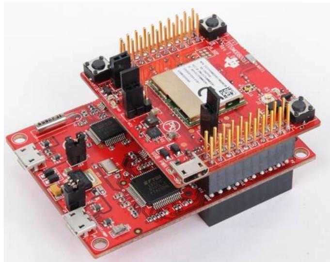
Figure 15. The CC3100BOOST Connected to the EMUBOOST
