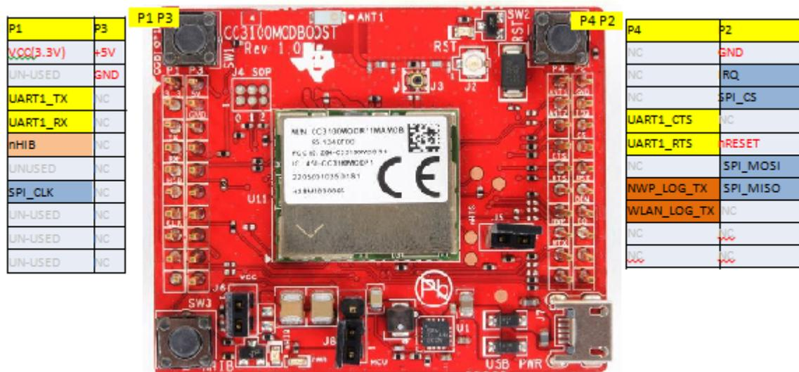
Figure 4. Signal Assignments
