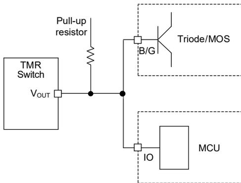
Figure 10. Application diagram for driving power load
