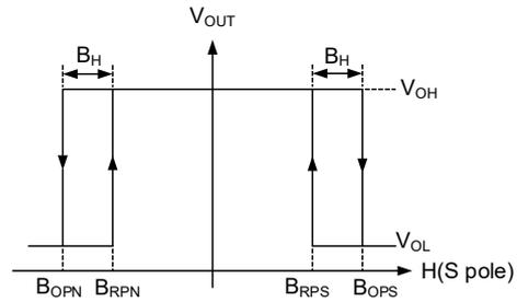
Figure 3. Switching characteristics
