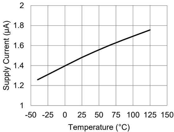
Figure 7. Supply current versus temperature ( $V_{CC} = 3\text{ V}$ )
