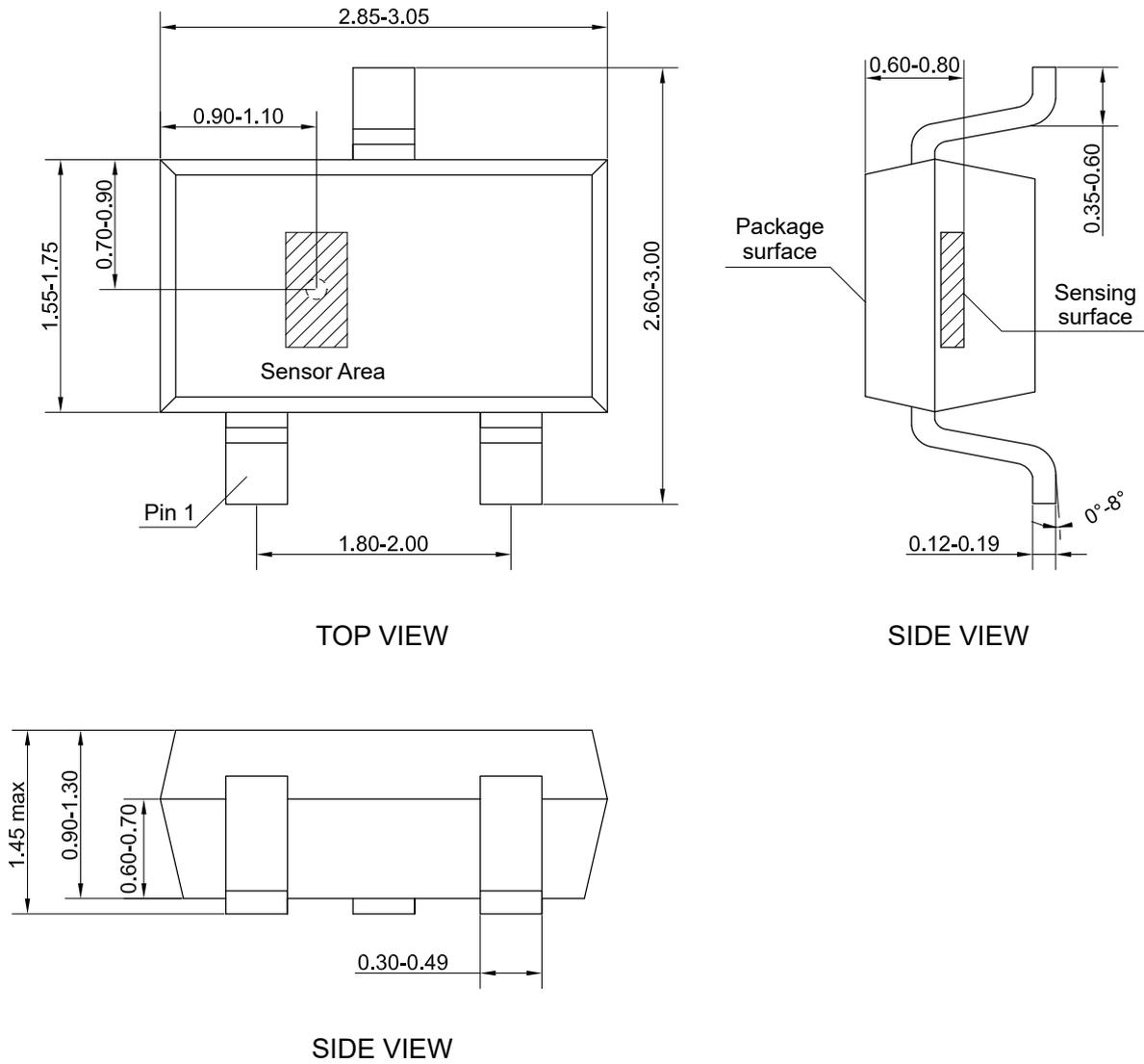
Figure 11. Package outline of SOT23-3 (unit: mm)
