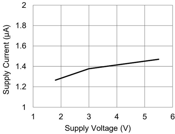
Figure 5. Supply current versus supply voltage ( $T_A=25^\circ\text{C}$ )
