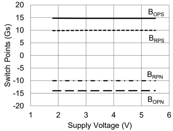
Figure 6. Switch points versus supply voltage ( $T_A=25^\circ\text{C}$ )
