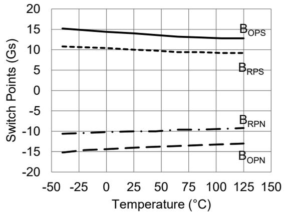
Figure 8. Switch points versus temperature ( $V_{CC} = 3\text{ V}$ )
