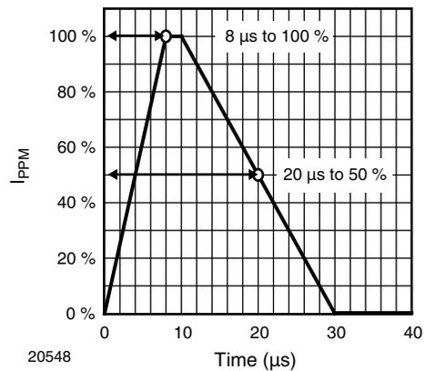
Fig. 2 - 8/20  $\mu s$  Peak Pulse Current Wave Form
