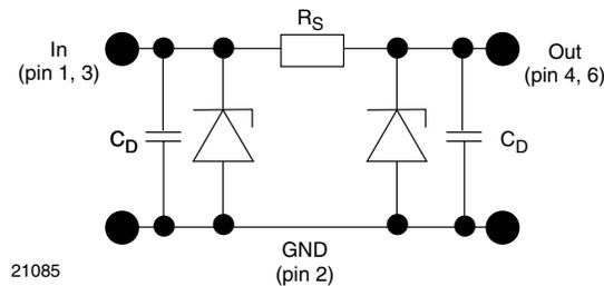
Each filter is symmetrical so that both ports can be used as input or output.
