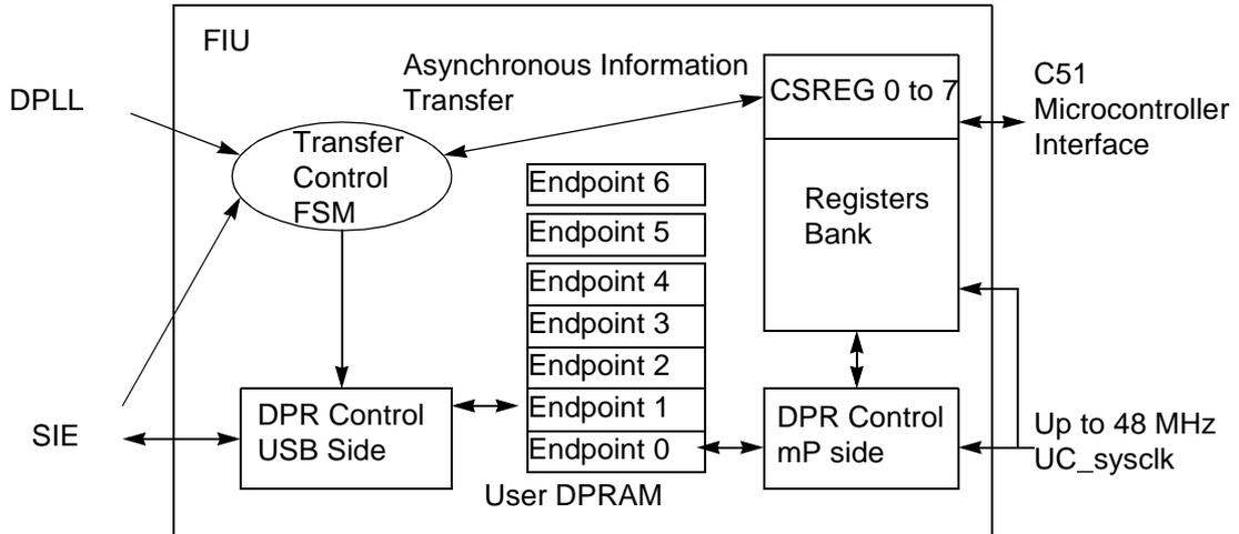
**Figure 56.** Minimum Intervention from the USB Device Firmware
