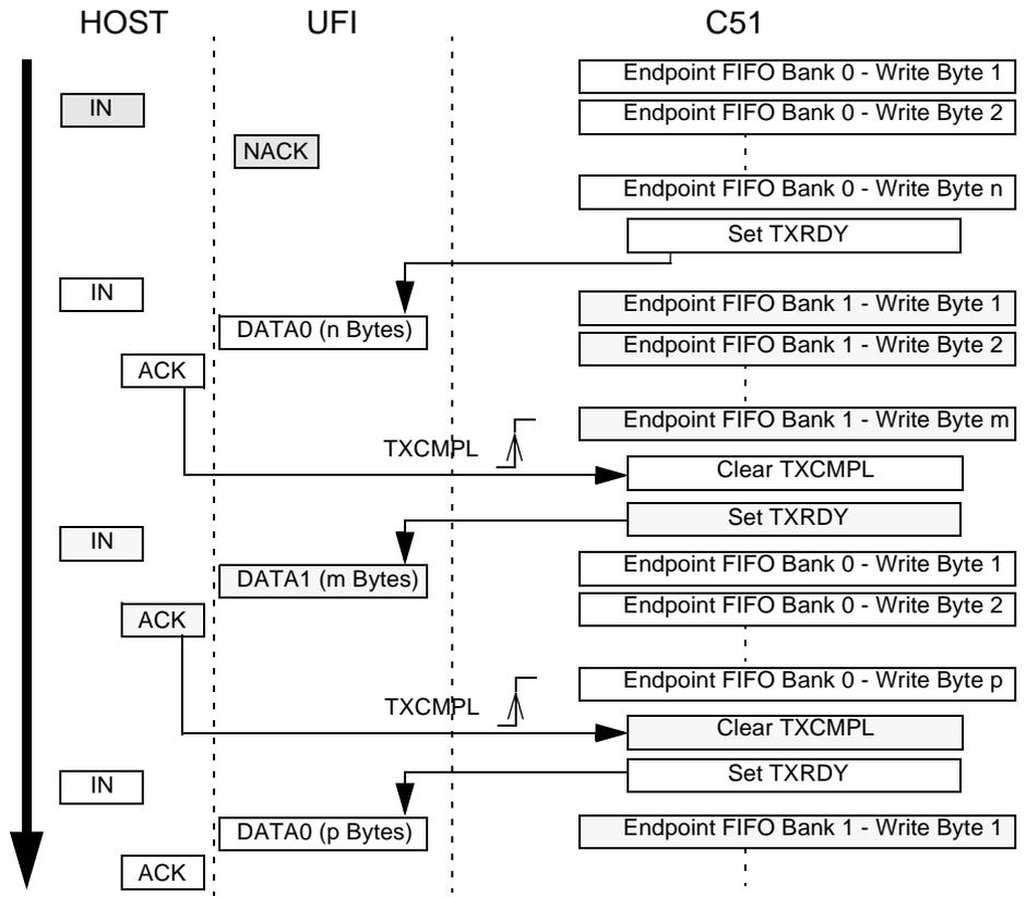
An endpoint will be first enabled and configured before being able to send Bulk or Interrupt packets.
