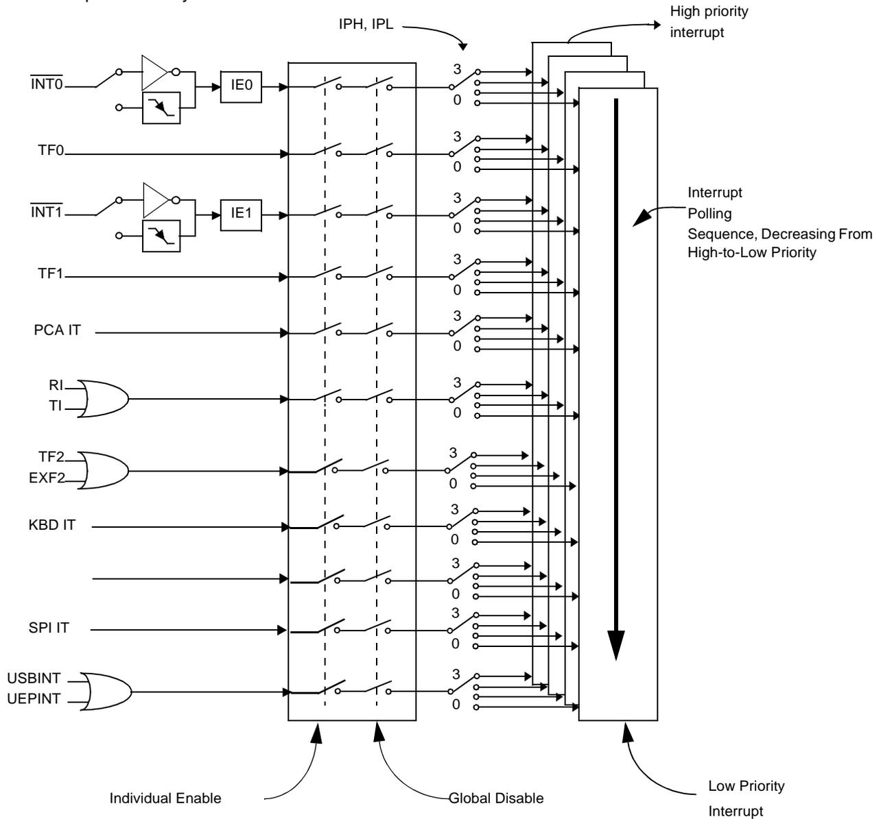
Each of the interrupt sources can be individually enabled or disabled by setting or clearing a bit in the Interrupt Enable register (Table 62). This register also contains a global disable bit, which must be cleared to disable all interrupts at once.
