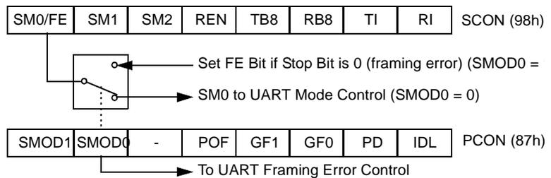
When this feature is enabled, the receiver checks each incoming data frame for a valid stop bit. An invalid stop bit may result from noise on the serial lines or from simultaneous transmission by two CPUs. If a valid stop bit is not found, the Framing Error bit (FE) in SCON register (See Table 57) bit is set.
