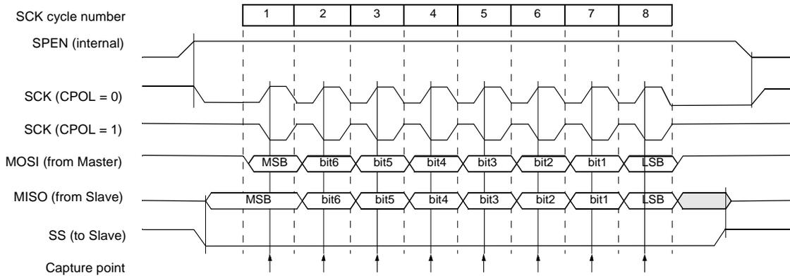
**Figure 43. Data Transmission Format (CPHA = 1)**
