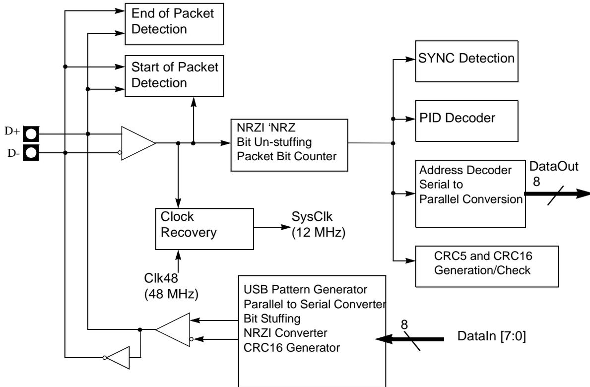
**Function Interface Unit (FIU)** The Function Interface Unit provides the interface between the AT89C5131 and the SIE. It manages transactions at the packet level with minimal intervention from the device firmware, which reads and writes the endpoint FIFOs.
