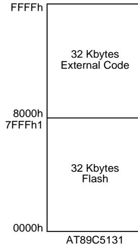
**Note:** If the program executes exclusively from on-chip code memory (not from external memory), beware of executing code from the upper byte of on-chip memory (7FFFh) and thereby disrupting I/O Ports 0 and 2 due to external prefetch. Fetching code constant from this location does not affect Ports 0 and 2.
