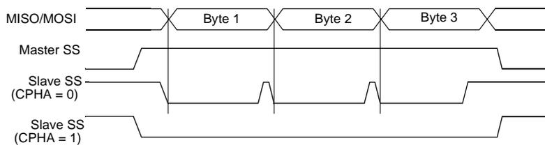
As shown in Figure 43, the first SCK edge is the MSB capture strobe. Therefore the Slave must begin driving its data before the first SCK edge, and a falling edge on the  $\overline{SS}$  pin is used to start the transmission. The  $\overline{SS}$  pin must be toggled high and then low between each byte transmitted (Figure 40).
