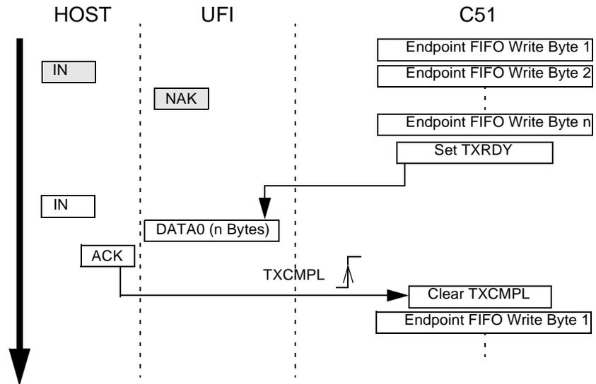
An endpoint will be first enabled and configured before being able to send Bulk or Interrupt packets.
