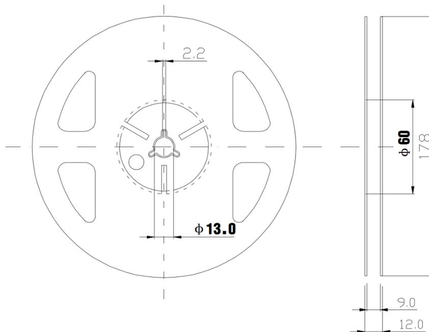
Unit: mm Tolerance: +/-0.15mm
