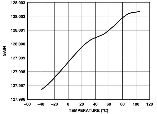
Figure 17. Gain Error (Gain = 128, Chop Disabled)
