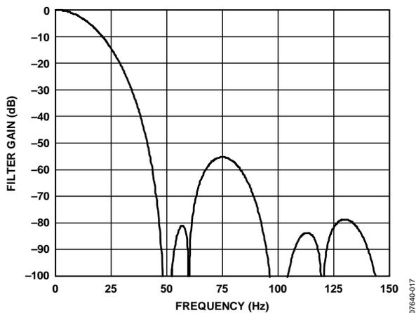
Figure 23. Sinc<sup>4</sup> Filter Response (50 Hz Output Data Rate, REJ60 = 1)
