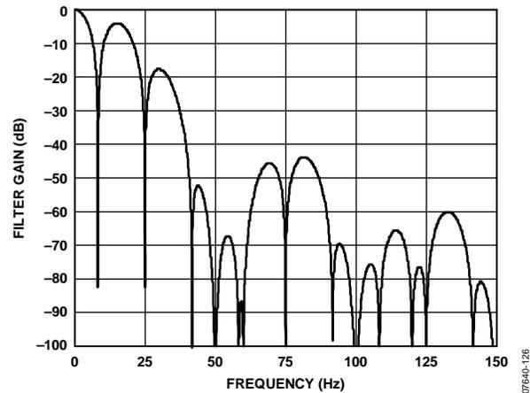
Figure 26. Sinc<sup>3</sup> Filter Response (16.7 Hz Output Data Rate, Chop Enabled, REJ60 = 1)
