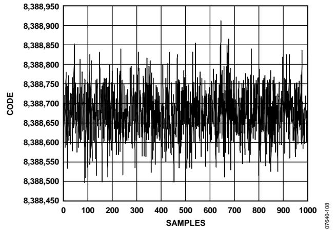
Figure 8. Noise ( $V_{REF} = 5\text{ V}$ , Output Data Rate = 4800 Hz, Gain = 128, Chop Disabled,  $Sinc^4$  Filter)
