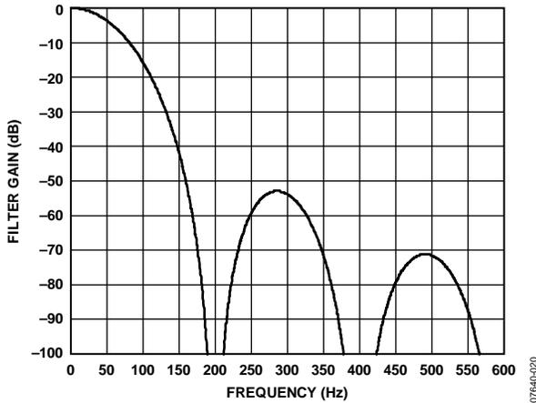
Figure 27. Sinc<sup>4</sup> Filter Response (50 Hz Output Data Rate, Zero Latency)
