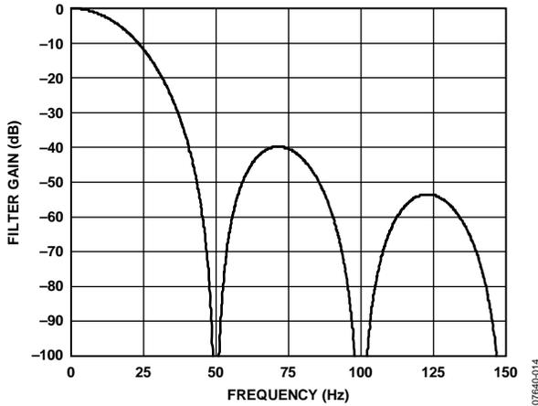
Figure 20. Sinc<sup>3</sup> Filter Response (50 Hz Output Data Rate)
