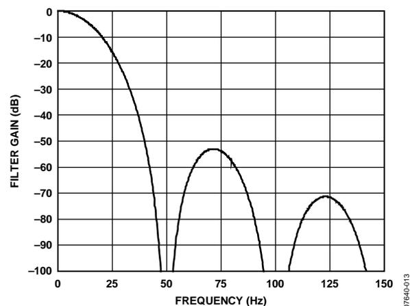
Figure 19.  $\text{Sinc}^4$  Filter Response (50 Hz Output Data Rate)
