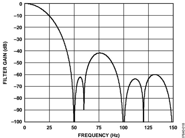
Figure 24. Sinc<sup>3</sup> Filter Response (50 Hz Output Data Rate, REJ60 = 1)
