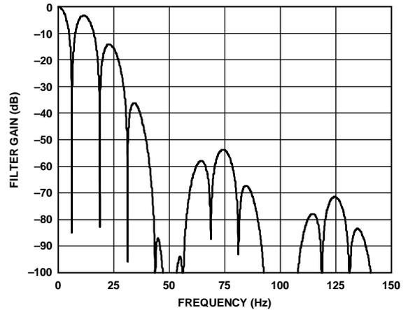
Figure 21. Sinc<sup>4</sup> Filter Response (Output Data Rate = 12.5 Hz, Chop Enabled)
