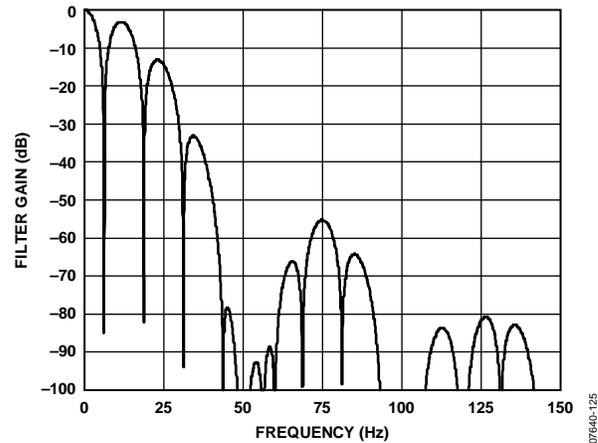
Figure 25. Sinc<sup>4</sup> Filter Response (12.5 Hz Output Data Rate, Chop Enabled, REJ60 = 1)
