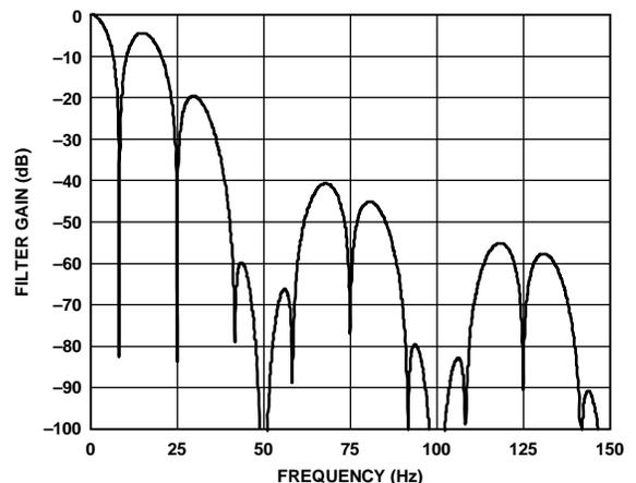
Figure 22. Sinc<sup>3</sup> Filter Response (Output Data Rate = 16.6 Hz, Chop Enabled)
