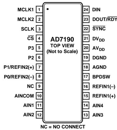
Figure 5. Pin Configuration
