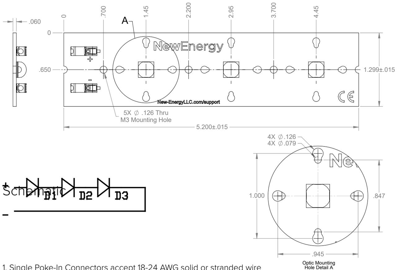
1. Single Poke-In Connectors accept 18-24 AWG solid or stranded wire
