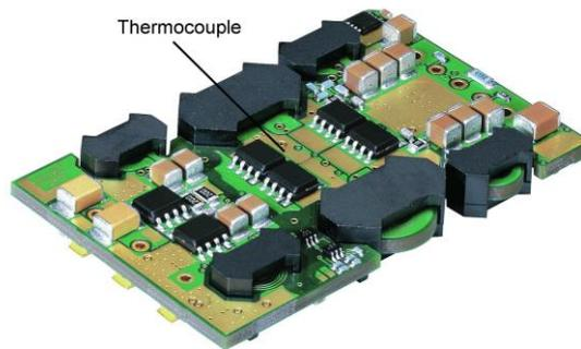
Figure 27. Location of the thermocouple for thermal testing.
