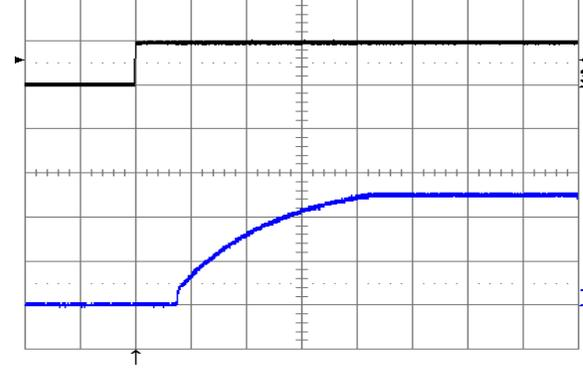
Figure 18. Turn-on transient at full rated load current (resistive) plus 10,000  $\mu\text{F}$  at  $V_{in} = 48\text{ V}$ , triggered via ON/OFF pin. Top trace: ON/OFF signal (5 V/div.). Bottom trace: output voltage (2 V/div.) Time scale: 2 ms/div.
