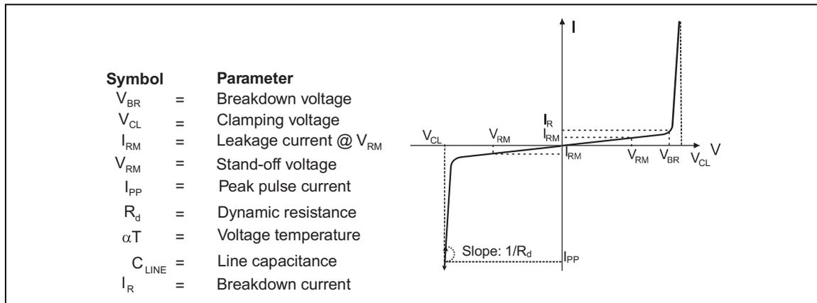
**Table 2. Electrical characteristics (values,  $T_{amb} = 25^{\circ}$  C)**
