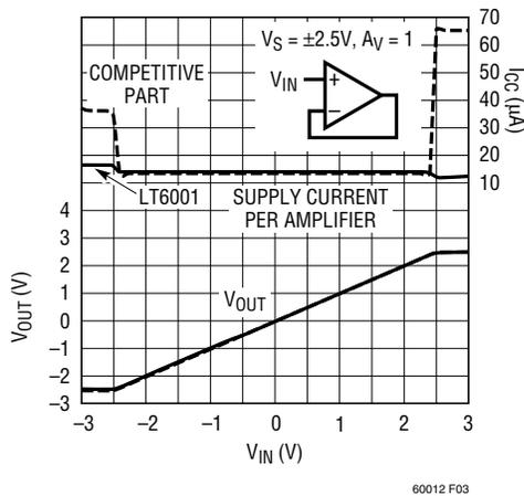
Figure 3.  $V_{OUT}$  and  $I_{CC}$  vs Input Voltage
