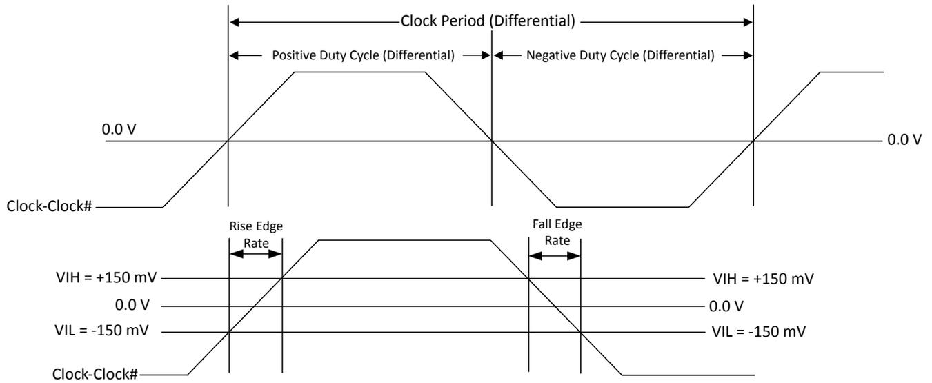
**Figure 6.2. Differential Output Signals (for AC Parameters Measurement)**
