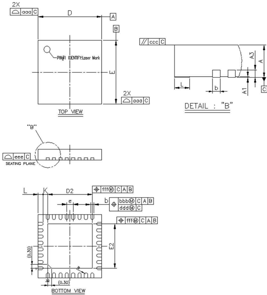
Figure 10.5. 32L 5 x 5 mm QFN Package Diagram
