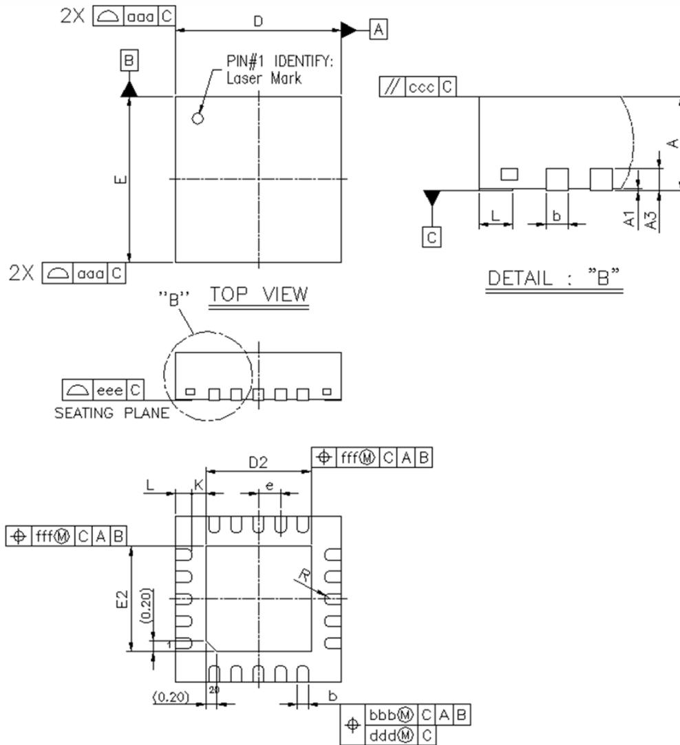
Figure 10.7. 20L 3 x 3 mm QFN Package Diagram
