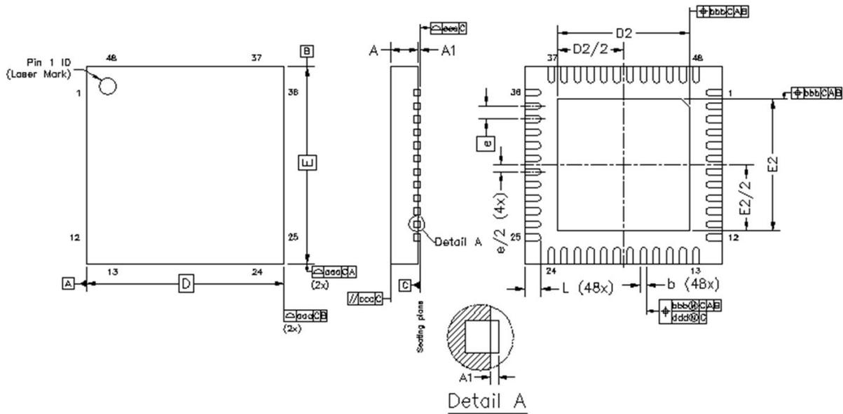
Figure 10.3. 48L 6 x 6 mm QFN Package Diagram
