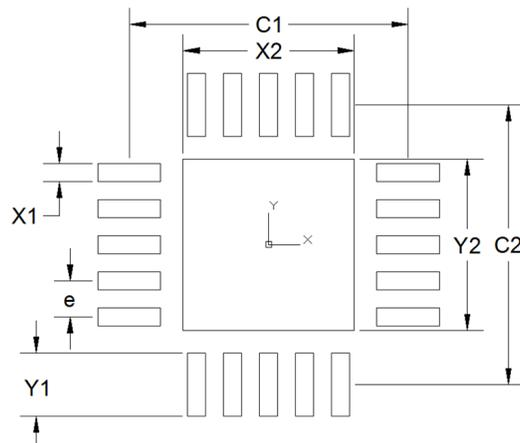
Figure 10.8. 20L 3 x 3 mm QFN Land Pattern
