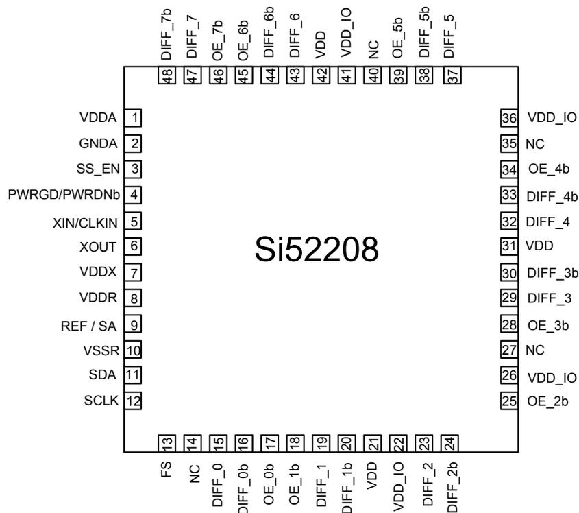
Figure 9.2. 48-pin QFN
