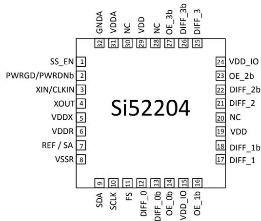
Figure 9.3. 32-pin QFN
