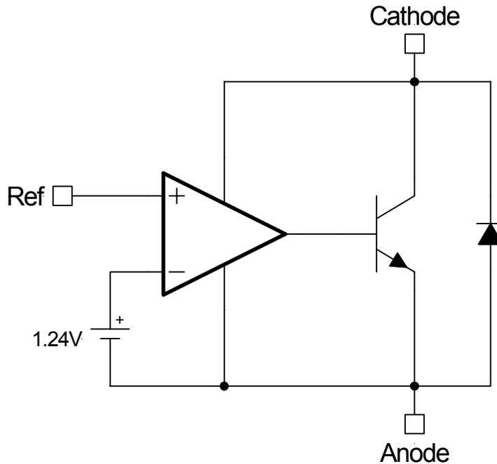
Figure 2 - Simplified block diagram of the IRU431L.
