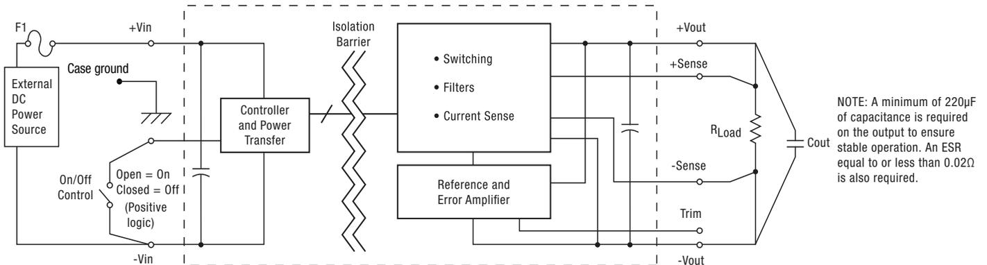
Figure 1. Simplified Schematic
