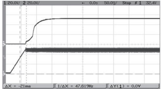
Step Load Transient Response (Vin=48V, Vout=nom, Cload=220uF, Iout=50-75-50% of full load (1As/us), Ta=+25°C)
