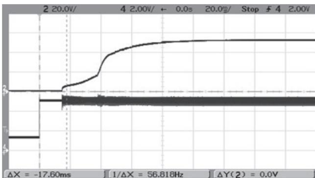
Start-up Delay (Vin=48V, Vout=nom, Iout=0A, Cload=220uF, Ta=+25°C)
