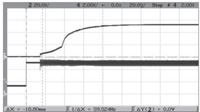
On/Off Enable Start-up (Vin=48V, Vout=nom, Iout=8.5A, Cload=1000uF, Ta=+25°C)
