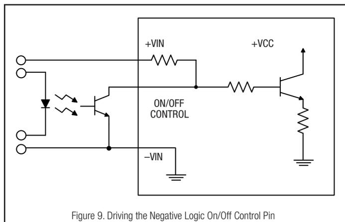
Figure 9. Driving the Negative Logic On/Off Control Pin
