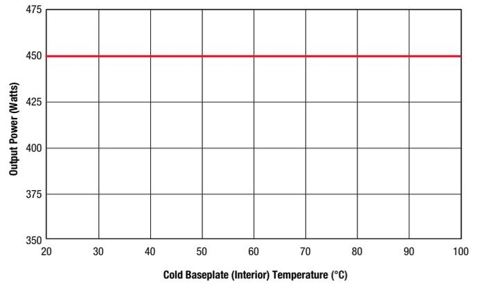
Maximum Current Temperature Derating at sea level (Vin=48V, transverse airflow, on 10" x 10" PCB with baseplate)
