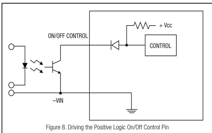
Figure 8. Driving the Positive Logic On/Off Control Pin
