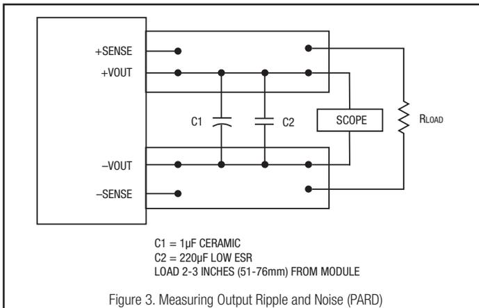
Figure 3. Measuring Output Ripple and Noise (PAR)
