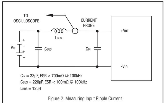
multiple external capacitors. Be sure to calculate component temperature rise from reflected AC current dissipated inside capacitor ESR. Our Application Engineers can recommend potential solutions.
