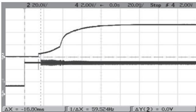
On/Off Enable Start-up (Vin=48V, Vout=nom, Iout=8.5A, Cload=220uF, Ta=+25°C)
