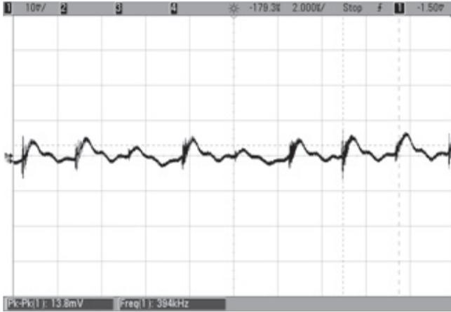
Output ripple and Noise (Vin=48V, Iout=8.5A, Cload=220uF, Ta=+25°C)
