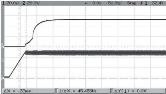
Start-up Delay (Vin=48V, Vout=nom, Iout=8.5A, Cload=1000uF, Ta=+25°C)
