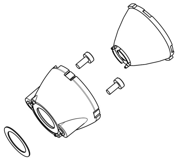
1. Place holder on PCB using the holder location pins as guide elements. Holder is fixed either by with on-board PU-tape or M3 screw with max 0.6Nm torque.
