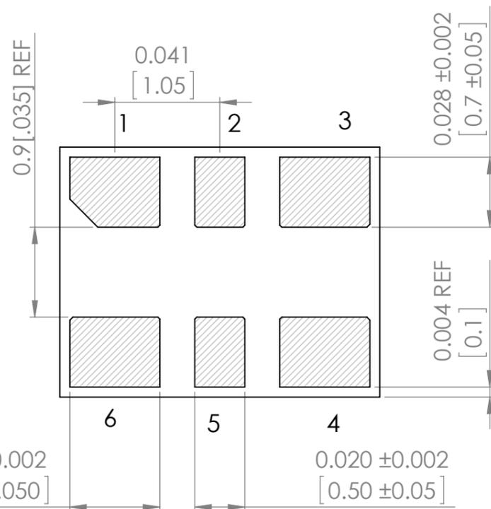
Note: Recommend using an approximately 0.01 uF bypass capacitor between PIN 6 and 3.
