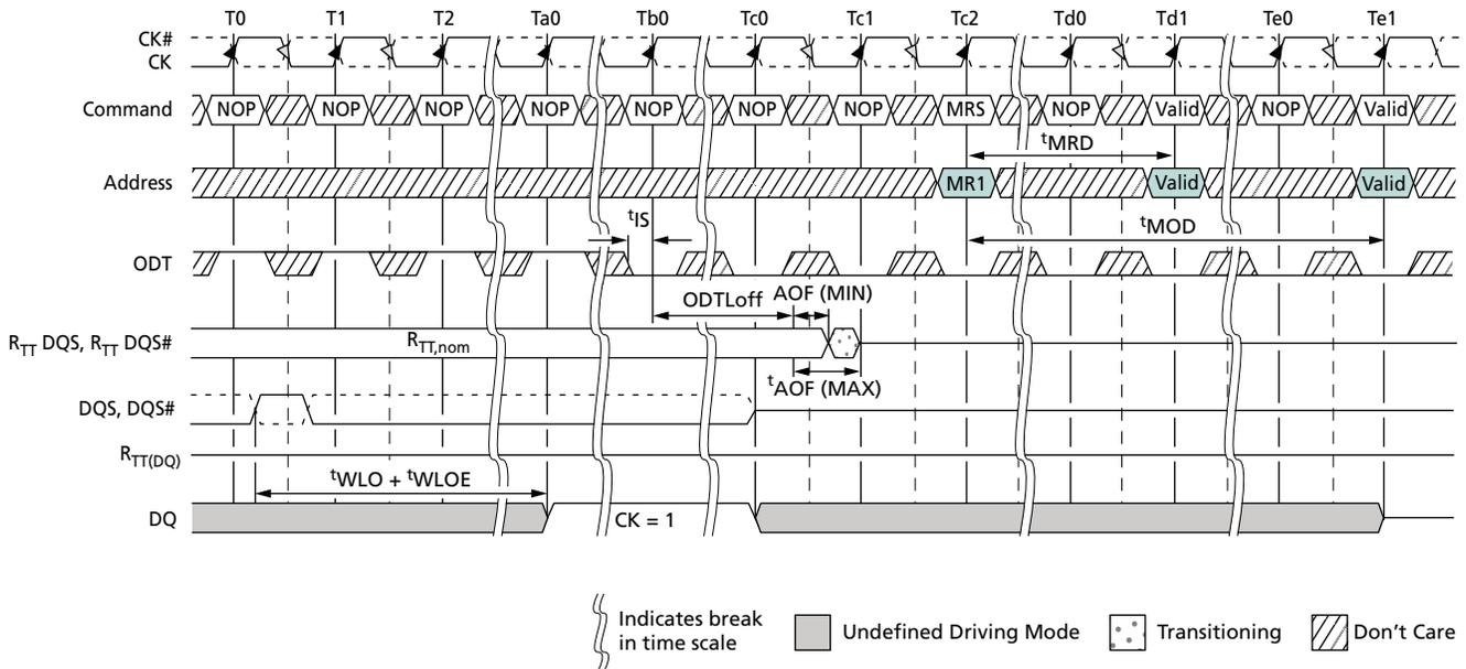
Note: 1. The DQ result, = 1, between Ta0 and Tc0, is a result of the DQS, DQS# signals capturing CK HIGH just after the T0 state.
