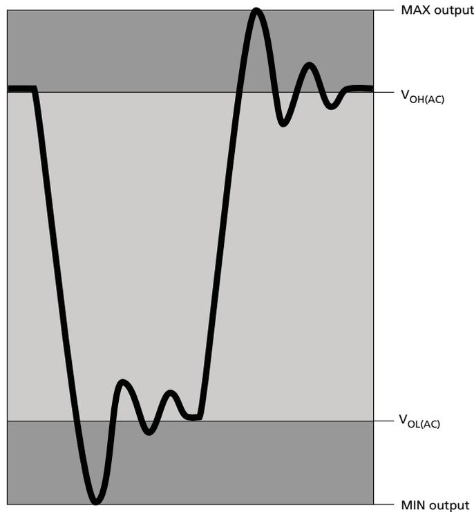
Figure 28: Differential Output Signal
