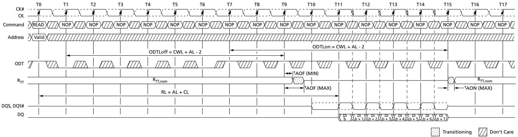
Note: 1. ODT must be disabled externally during READs by driving ODT LOW. For example, CL = 6; AL = CL - 1 = 5; RL = AL + CL = 11; CWL = 5; ODTL<sub>on</sub> = CWL + AL - 2 = 8; ODTL<sub>off</sub> = CWL + AL - 2 = 8. R<sub>TT,nom</sub> is enabled. R<sub>TT(WR)</sub> is a "Don't Care."
