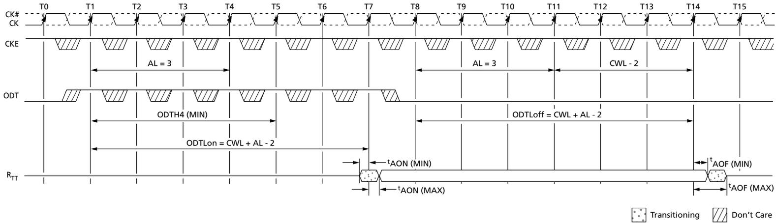
Note: 1. AL = 3; CWL = 5; ODTLon = WL = 6.0; ODTLoff = WL - 2 = 6. R<sub>TT,nom</sub> is enabled.
