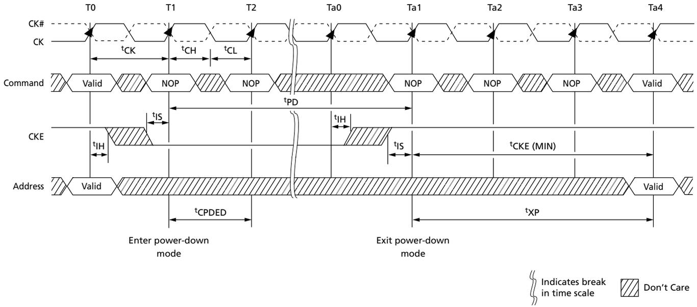
Figure 96: Precharge Power-Down (Fast-Exit Mode) Entry and Exit
