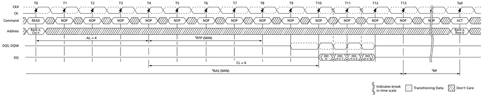
DQS to DQ output timing is shown in Figure 76 (page 164). The DQ transitions between valid data outputs must be within  $t_{DQSQ}$  of the crossing point of DQS, DQS#. DQS must also maintain a minimum HIGH and LOW time of  $t_{QSH}$  and  $t_{QSL}$ . Prior to the READ preamble, the DQ balls will either be floating or terminated, depending on the status of the ODT signal.
