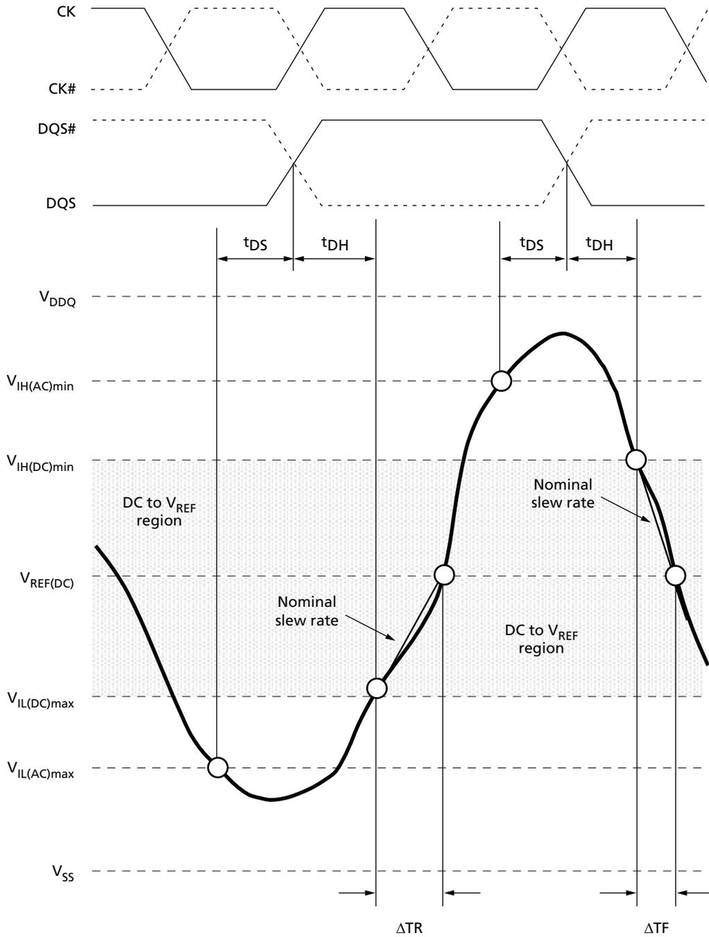
$$\text{Hold slew rate rising signal} = \frac{V_{REF(DC)} - V_{IL(DC)max}}{\Delta TR}$$
