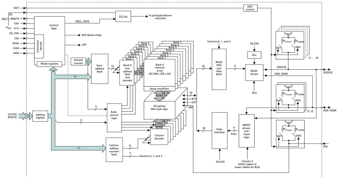
**Figure 4: 256 Meg x 8 Functional Block Diagram**
