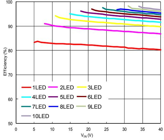
**Efficiency vs.  $V_{IN}$  ( $L1=33\mu H$ ,  $R_s=0.1\Omega$ )**
