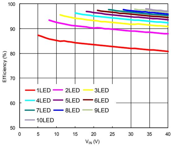
**Efficiency vs.  $V_{IN}$  ( $L1=47\mu H$ ,  $R_s=0.15\Omega$ )**
