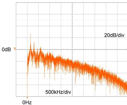
**Fixed Switching Frequency Waveform Spectrum of Competitor**
