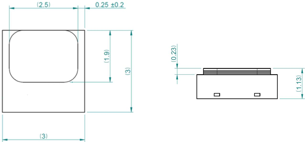
Dimensions are given in mm, tolerances are  $\pm 0.1$ mm. The die pad (thermal center pad) is internally connected to GND.
