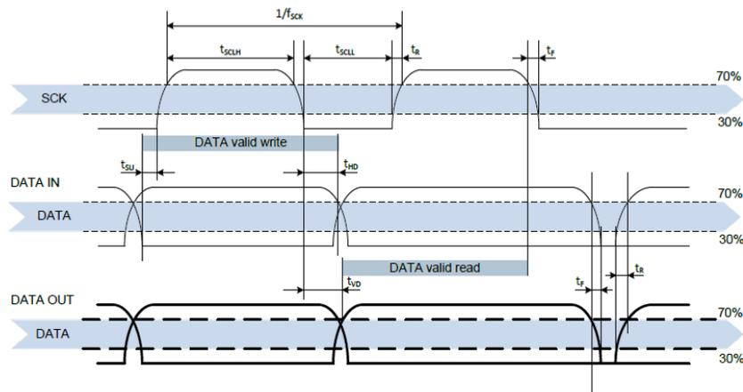
DATA directions are seen from the HTU21D(F) sensor. DATA line in bold is controlled by the sensor. DATA valid read time is triggered by falling edge of anterior toggle.
