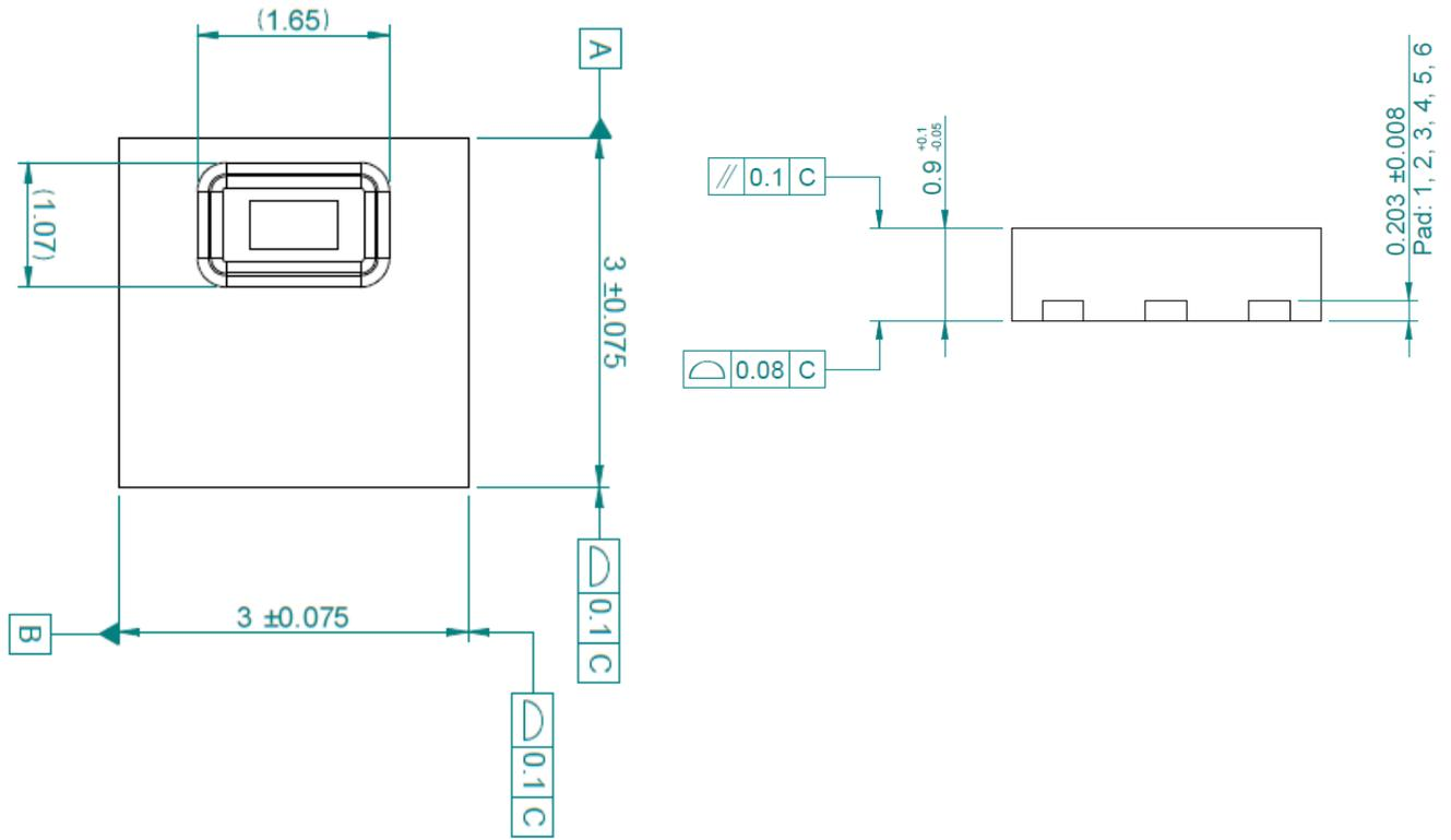
Dimensions are given in mm, tolerances are ±0.1mm. The die pad (thermal center pad) is internally connected to GND.
