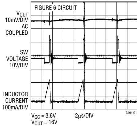
**LT3494A Switching Waveforms at 30mA Load**
