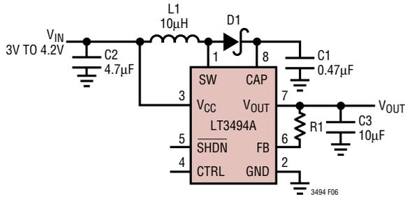
C1, C2: X5R OR X7R WITH SUFFICIENT VOLTAGE RATING
