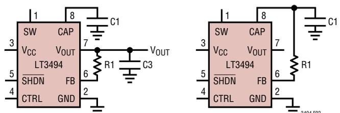
**Figure 2. Feedback Connection Using the CAP Pin or the V<sub>OUT</sub> Pin**
