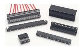
The .400"/10.0mm ELL product line is a doublespaced version of Amphenol Pcd's broad family of .200"/5.0mm ELF plugs and headers, offering a higher voltage rating—600Vrms—and the same range of configurations and accessories as the ELF line shown on pages 22 and 23.
