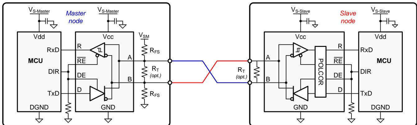
Figure 11. Point-To-Point Data Link With Cross-Wire Fault
