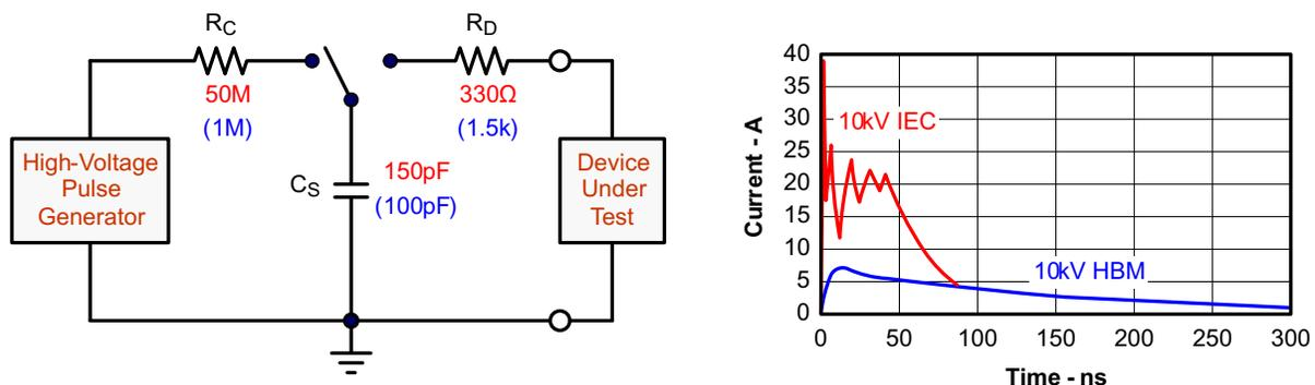
Figure 16. HBM and IEC-ESD Models and Currents in Comparison (HBM Values in Parenthesis)
