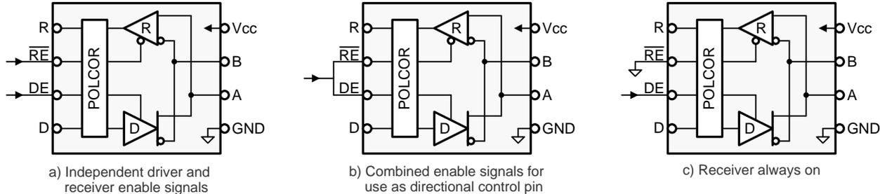
Figure 13. Transceiver Configurations
