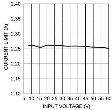
Figure 8. Current Limit vs  $V_{IN}$ , LM3406HV/LM3406HV-Q1
