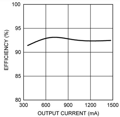
Figure 2. Efficiency Vs. Output Current (1)
