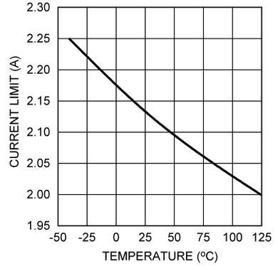
Figure 6. Current Limit vs Temperature
