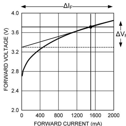
Calculating r<sub>D</sub> from the V<sub>F</sub> vs. I<sub>F</sub> Curve
