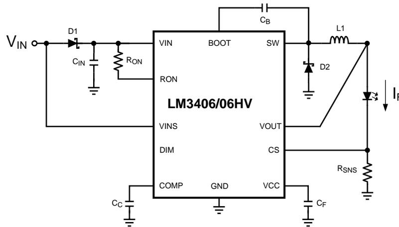
Typical Application using Two-Wire Dimming
