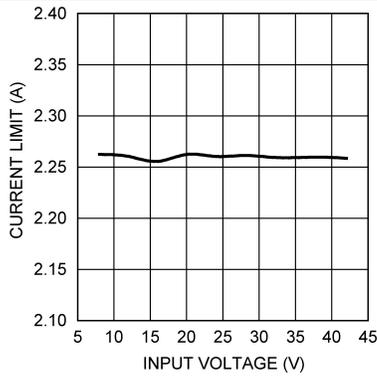
Figure 7. Current Limit vs  $V_{IN}$ , LM3406
