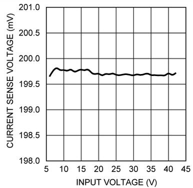
Figure 4.  $V_{REF}$  vs  $V_{IN}$ , LM3406
