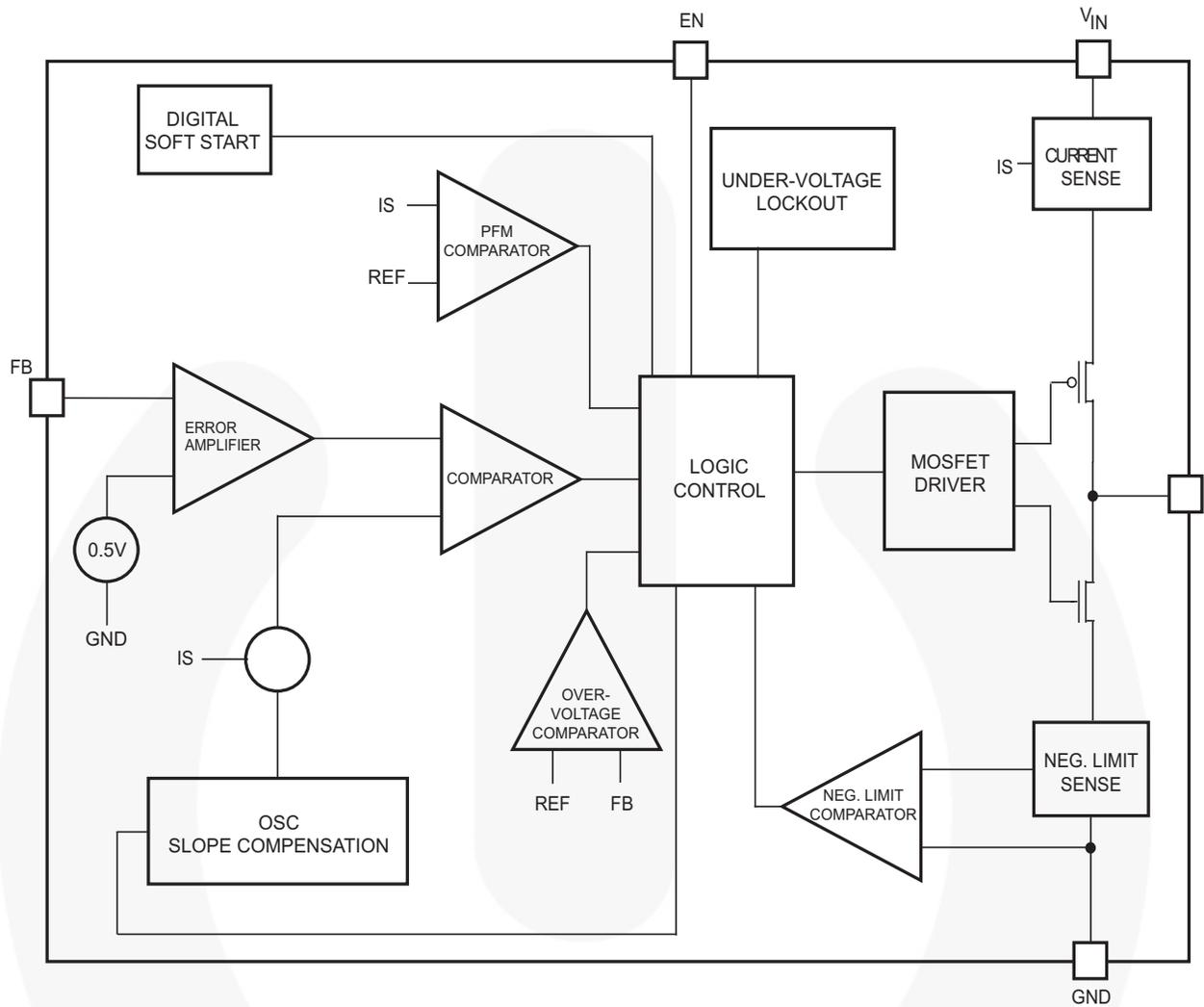
Figure 15. Block Diagram
