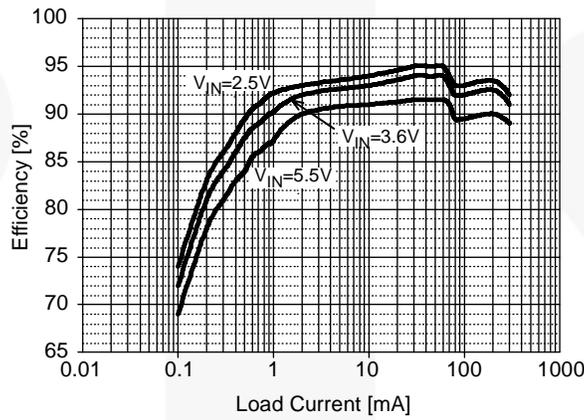
Figure 3. Efficiency vs. Load Current ( $V_{OUT}=1.8V$ )
