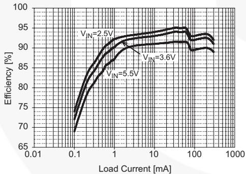
Figure 11. Efficiency vs. Load Current ( $V_{OUT}=1.8\text{V}$ )
