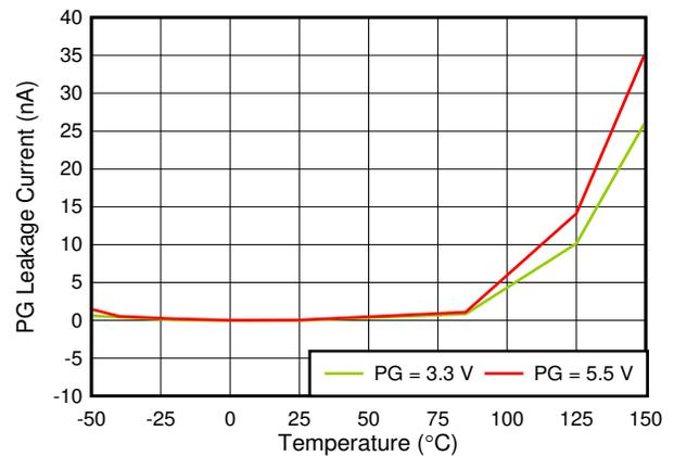
Figure 6-16.  $I_{kg(PG)}$  vs Temperature and PG Pin Voltage
