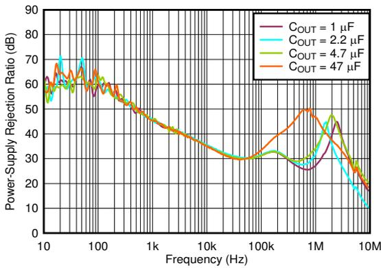
$V_{IN} = 3.8\text{ V}$ ,  $V_{OUT} = 3.3\text{ V}$ ,  $I_{OUT} = 500\text{ mA}$
