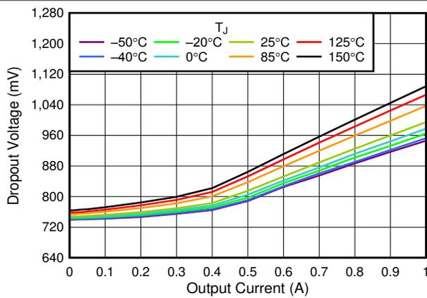
Figure 6-5. 0.55-V Dropout Voltage vs  $I_{OUT}$
