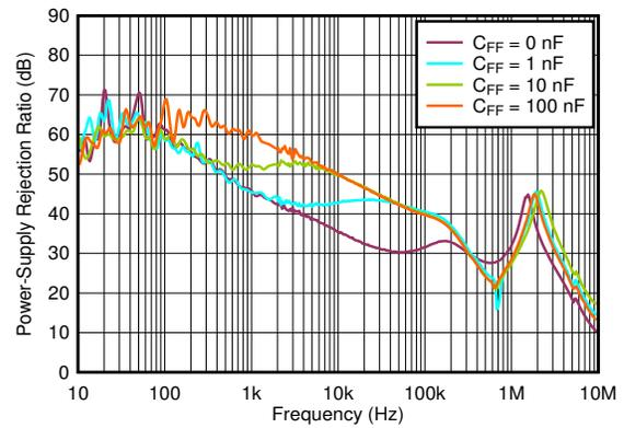
$V_{IN} = 3.8\text{ V}$ ,  $V_{OUT} = 3.3\text{ V}$ ,  $I_{OUT} = 500\text{ mA}$
