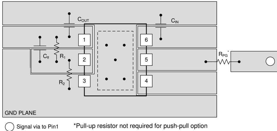
**Figure 10-1. Layout Example for the DRV Package**
