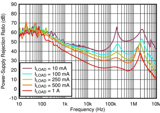
$V_{IN} = 3.8\text{ V}$ ,  $V_{OUT} = 3.3\text{ V}$ ,  $C_{OUT} = 2.2\ \mu\text{F}$
