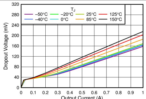
Figure 6-6. 5.5-V Dropout Voltage vs  $I_{OUT}$
