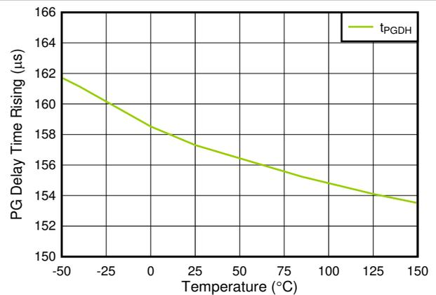
Figure 6-18.  $t_{PGDH}$  vs Temperature
