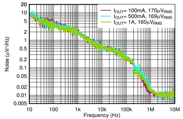
$V_{IN} = 3.8\text{ V}$ ,  $V_{OUT} = 3.3\text{ V}$ ,  $C_{OUT} = 4.7\ \mu\text{F}$ ,  $V_{RMS}\text{ BW} = 10\text{ Hz to }100\text{ kHz}$
