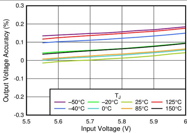
$V_{OUT} = 5.5\text{ V}$ ,  $I_{OUT} = 1\text{ mA}$
