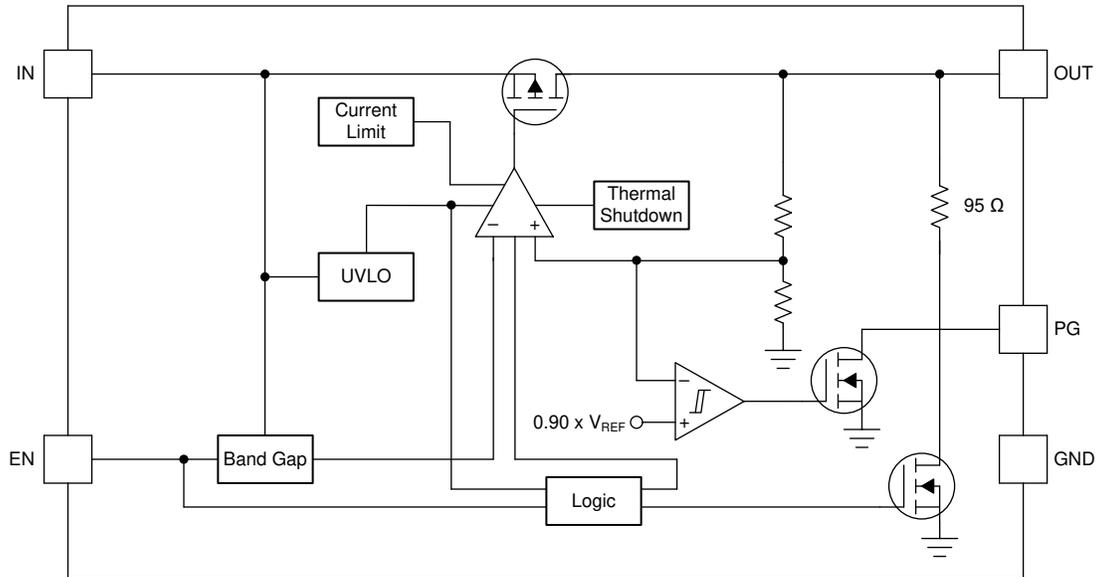
**Figure 7-3. Fixed Voltage Version With Open-Drain Power-Good**
