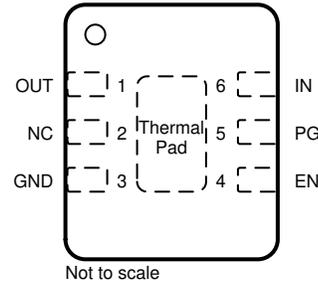
**Figure 5-2. DRV Package, 6-Pin Fixed WSON (Top View)**
