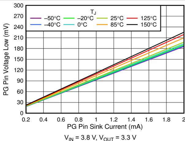
Figure 6-17.  $V_{OL(PG)}$  vs PG Pin Sink Current
