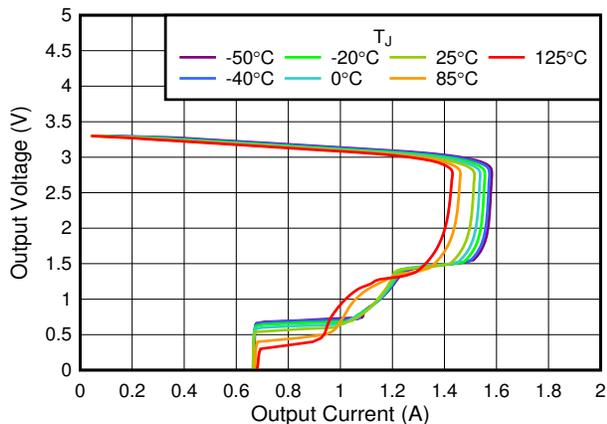
Figure 6-23. 3.3-V Foldback Current Limit vs  $I_{OUT}$
