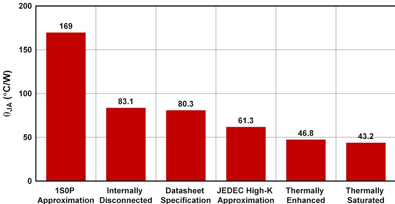
**Figure 8-8. TPS746-Q1 (WSON)  $R_{\theta JA}$  vs Board Layout**
