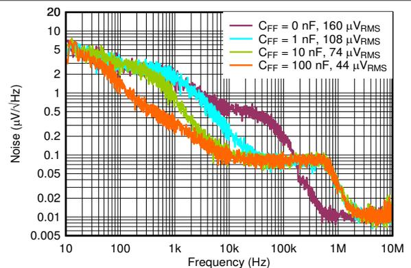
$V_{IN} = 3.8\text{ V}$ ,  $V_{OUT} = 3.3\text{ V}$ ,  $I_{OUT} = 500\text{ mA}$ ,  $C_{OUT} = 2.2\ \mu\text{F}$ ,  $V_{RMS}\text{ BW} = 10\text{ Hz to }100\text{ kHz}$
