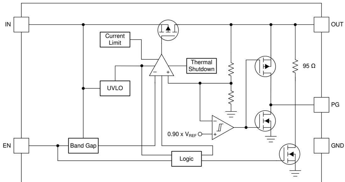
**Figure 7-4. Fixed Voltage Version With Push-Pull Power-Good**
