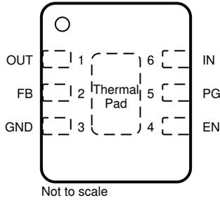
**Figure 5-1. DRV Package, 6-Pin Adjustable WSON (Top View)**
