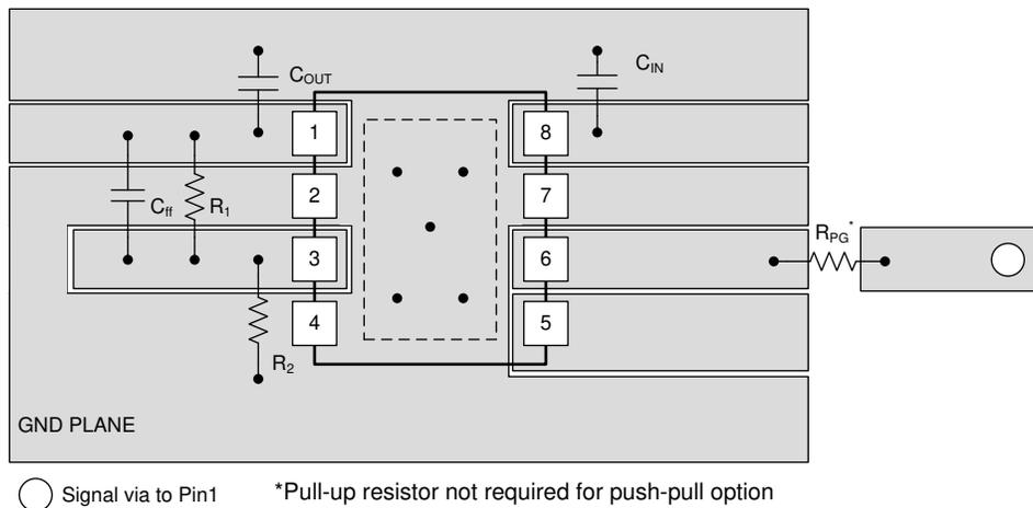
**Figure 10-2. Layout Example for the DRB package**
