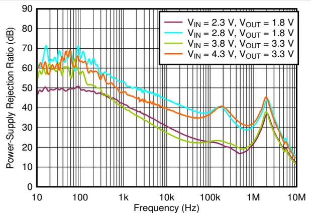
$I_{OUT} = 1\text{ A}$ ,  $C_{OUT} = 2.2\text{ }\mu\text{F}$
