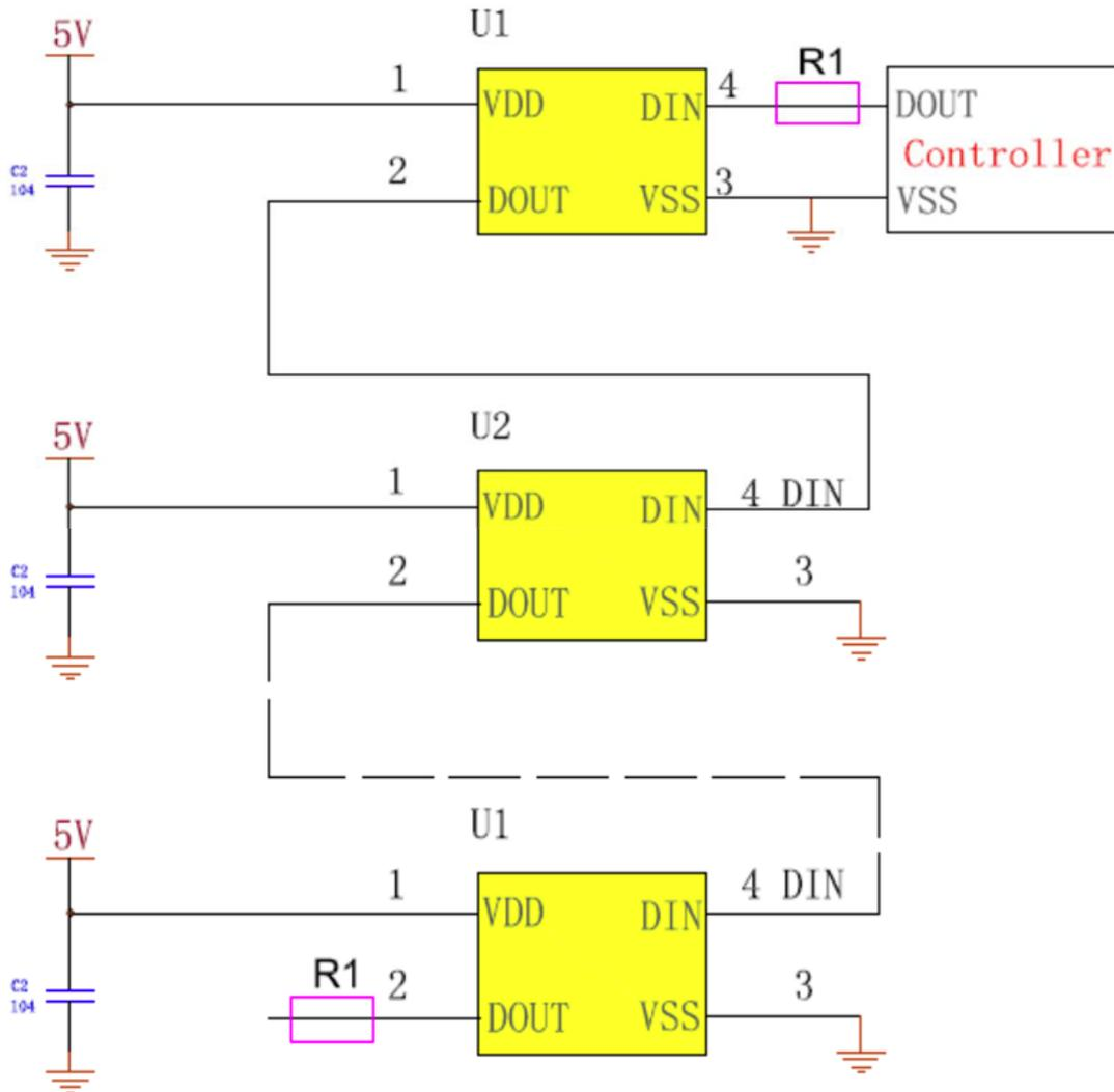
Product signal input and output must be connected in series with protection resistor R1. R1 depends on the size of the cascade amount, the greater the number of cascade, the smaller R1. The general recommended value is between 200-2K $\Omega$ , usually the recommended value is typical 500 $\Omega$ .
