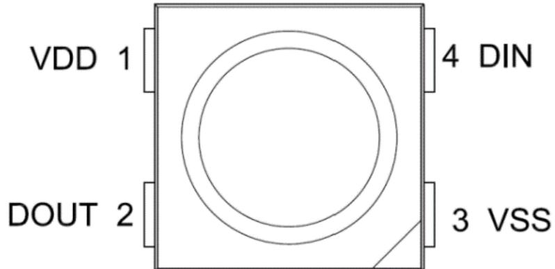
Figure 2. IN- PI55QATPRGPBPW-XX Pin Configuration
