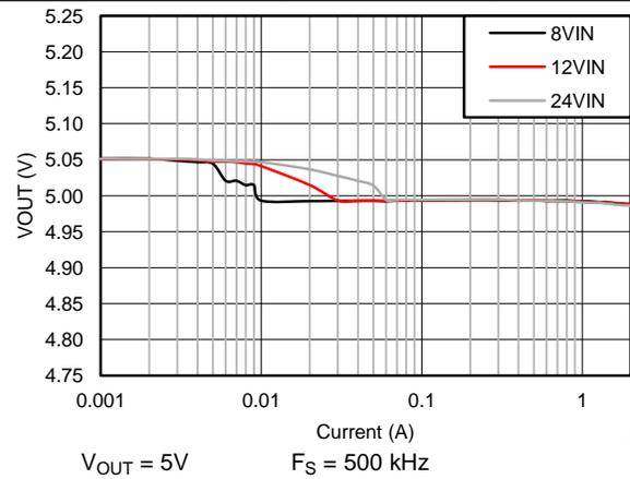
Figure 8.  $V_{OUT}$  Regulation
