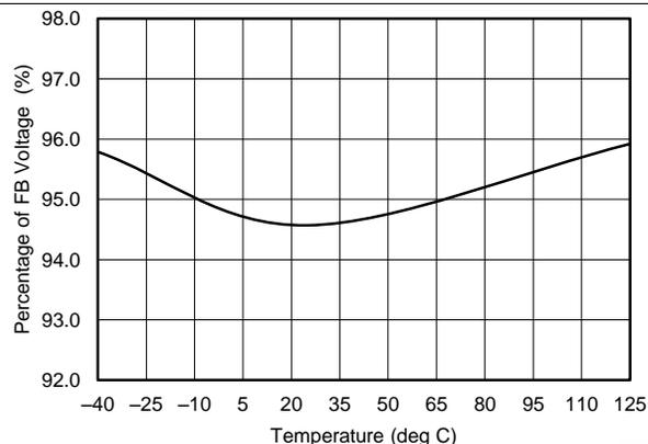
**Figure 24. PGOOD UVP Rising Threshold vs Junction Temperature**
