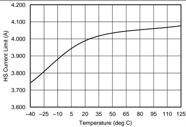
Figure 17. HS Current Limit vs Junction Temperature
