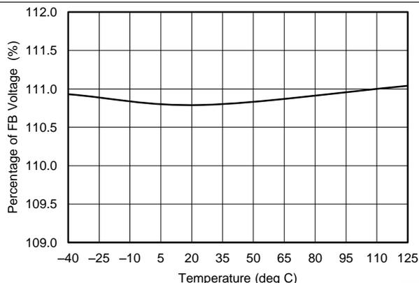
**Figure 21. PGOOD Falling Threshold vs Junction Temperature**
