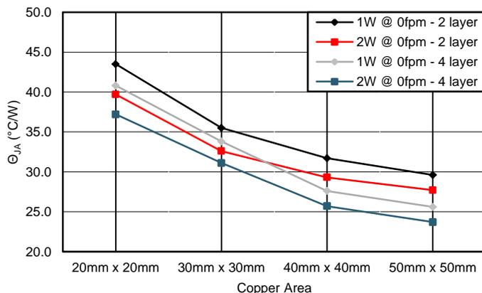
Figure 64.  $R_{\theta JA}$  vs Copper Area
