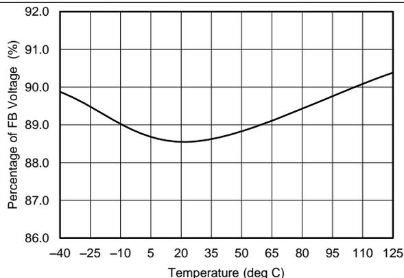
**Figure 23. PGOOD UVP Falling Threshold vs Junction Temperature**
