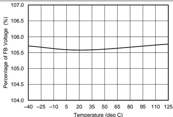
**Figure 22. PGOOD OVP Rising Threshold vs Junction Temperature**
