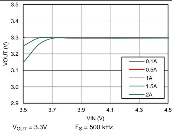
Figure 9. Dropout Curve
