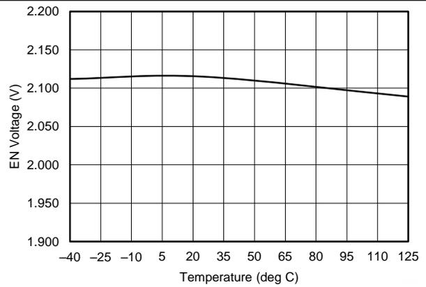
Figure 14. EN Rising Threshold vs Junction Temperature
