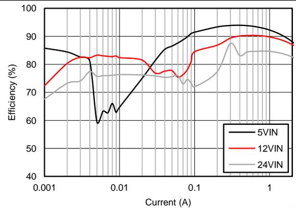
$V_{OUT} = 3.3V$   $F_S = 500\text{ kHz}$
