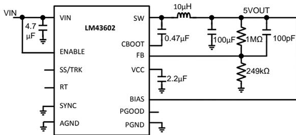
$V_{OUT} = 5V$        $F_S = 500\text{ kHz}$
