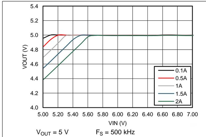
**Figure 57. Dropout Voltage**
