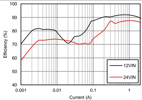
$V_{OUT} = 5V$        $F_S = 500\text{ kHz}$
