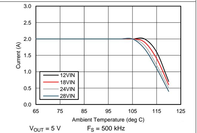
**Figure 62. Derating Curve**
