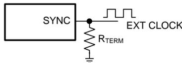
Figure 32. Frequency Synchronization
