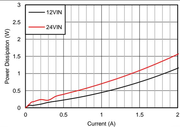
$V_{OUT} = 5V$        $F_S = 500\text{ kHz}$
