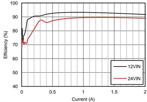
$V_{OUT} = 5V$        $F_S = 500\text{ kHz}$
