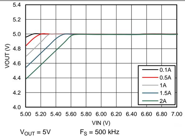
Figure 10. Dropout Curve
