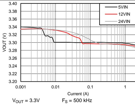
Figure 7.  $V_{OUT}$  Regulation
