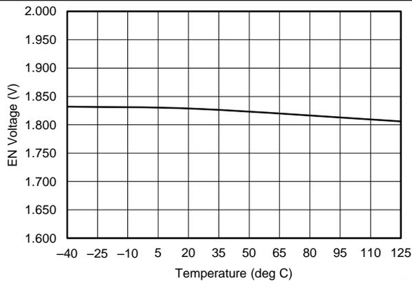
Figure 13. EN Falling Threshold vs Junction Temperature
