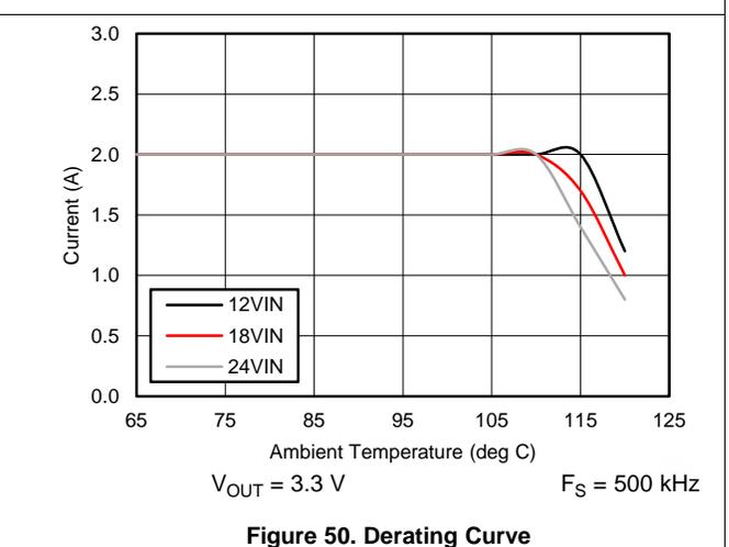
Unless otherwise specified,  $V_{IN} = 12V$ ,  $V_{OUT} = 3.3V$ ,  $F_S = 500\text{ kHz}$ . Please refer to [Application Performance Curves](#) for Bill of materials for each  $V_{OUT}$  and  $F_S$  combination.
