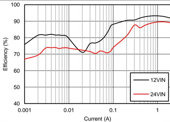
$V_{OUT} = 5V$        $F_S = 500\text{ kHz}$
