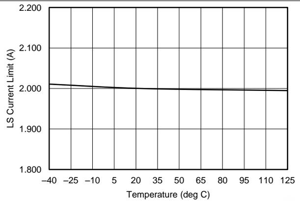
Figure 18. LS Current Limit vs Junction Temperature
