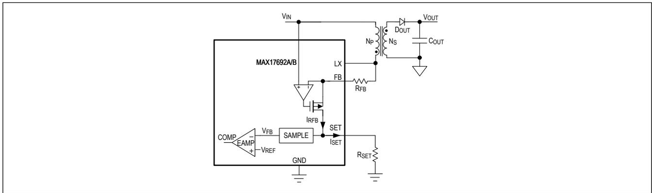
Figure 6. Simplified diagram of No-Opto Flyback Operation
