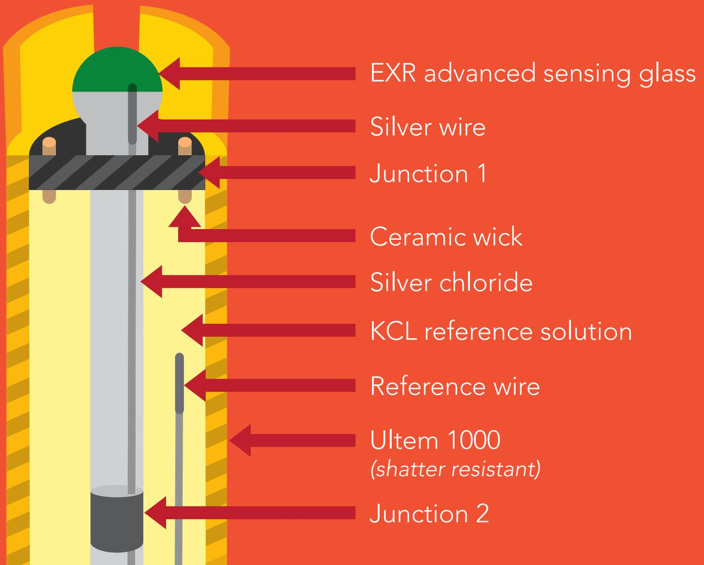
A pH electrode is a passive device that detects a current generated from hydrogen ion activity. This current (*which can be positive or negative*) is very weak and cannot be detected with a multimeter, or an analog to digital converter. This weak electrical signal can easily be disrupted and care should be taken to only use proper connectors and cables.
