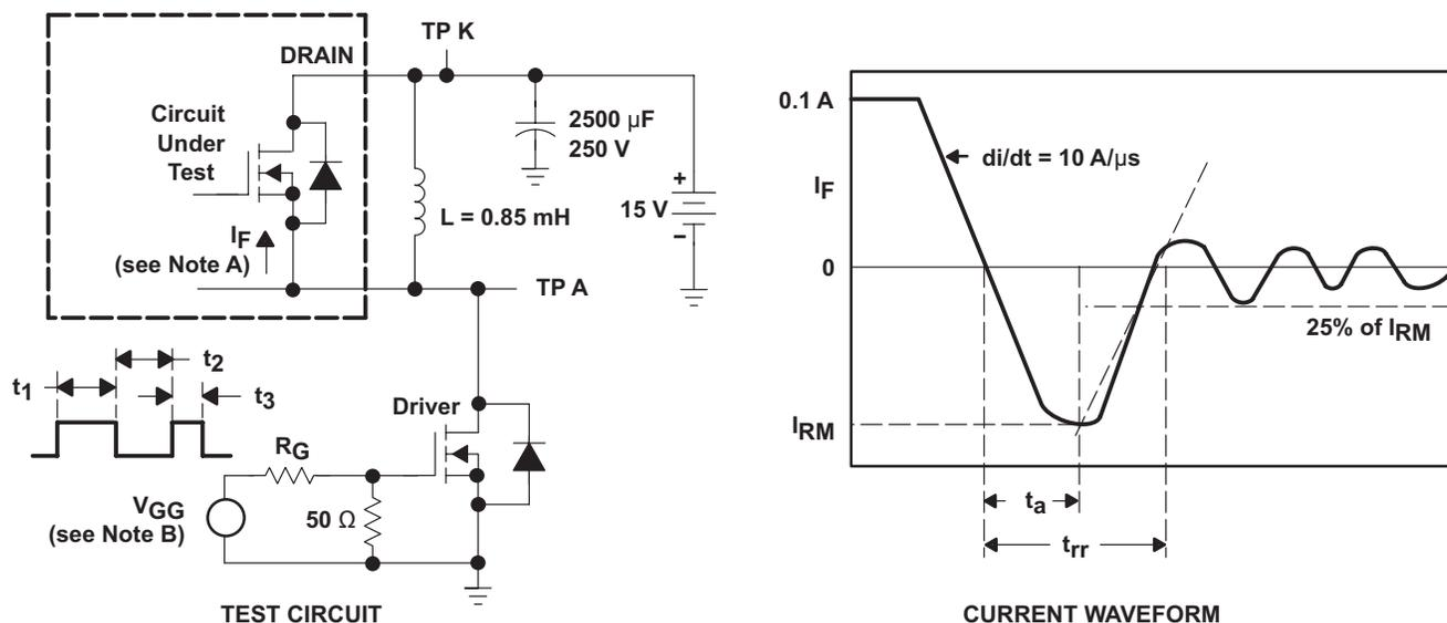
Figure 10. Reverse-Recovery-Current Test Circuit and Waveforms of Source-to-Drain Diode
