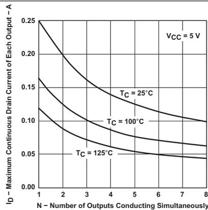
Figure 6. Maximum Continuous Drain Current of Each Output vs Number of Outputs Conducting Simultaneously
