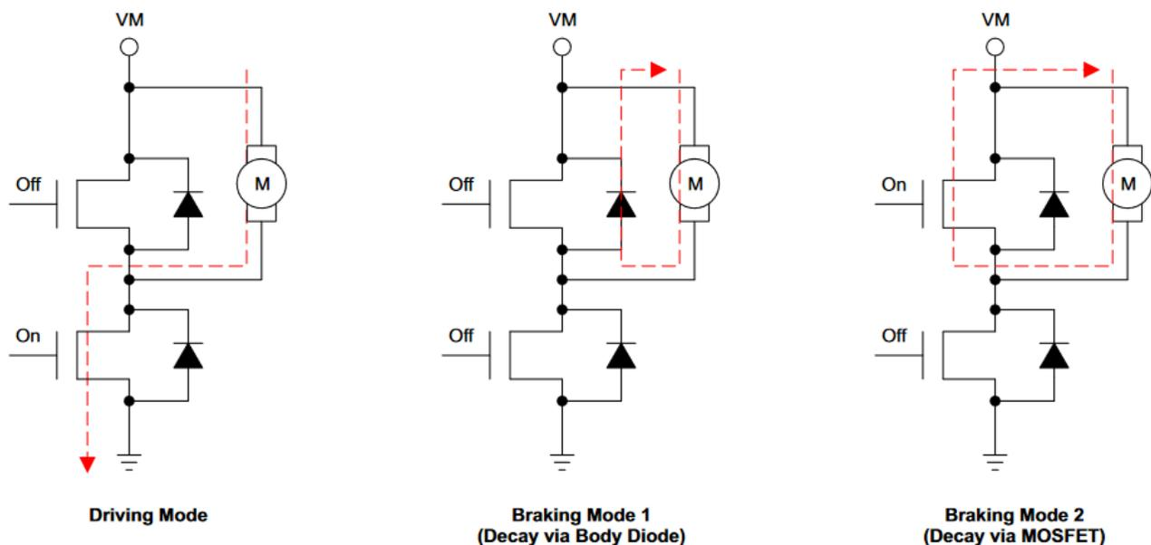
**Figure 7-4. Normal Driving and Current Decay Modes**
