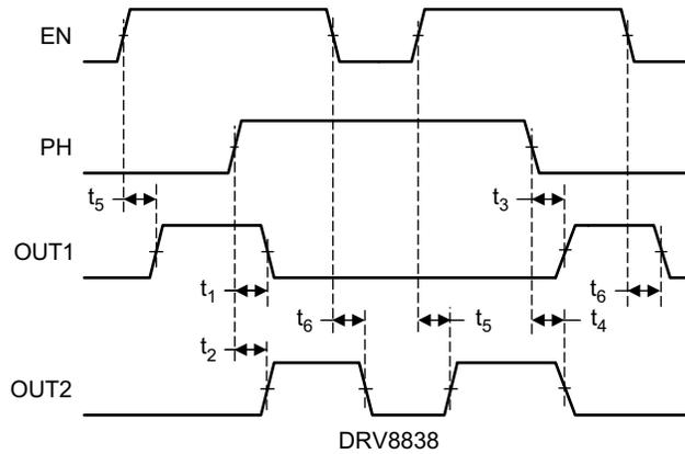
**Figure 6-1. Input and Output Timing for DRV8838**
