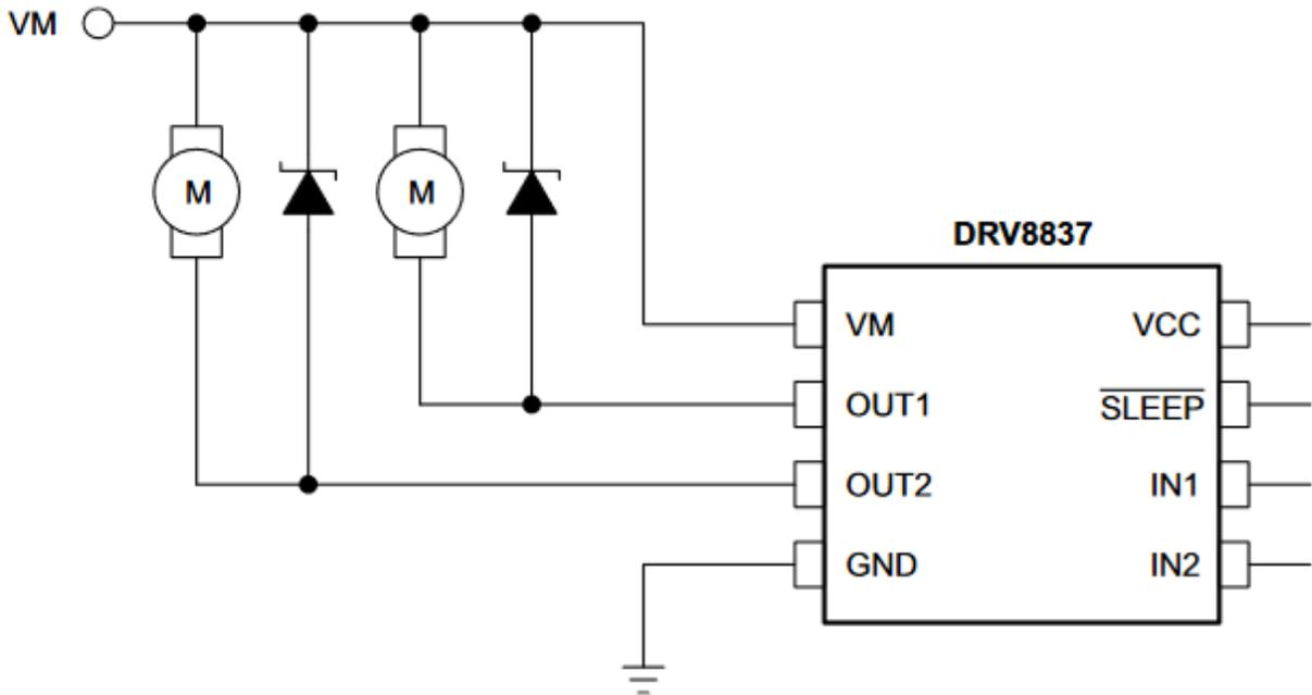
Figure 7-6. Improved Application Circuit for Better Motor Performance
