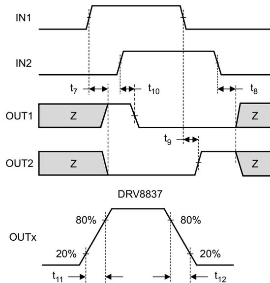
**Figure 6-2. Input and Output Timing for DRV8837**
