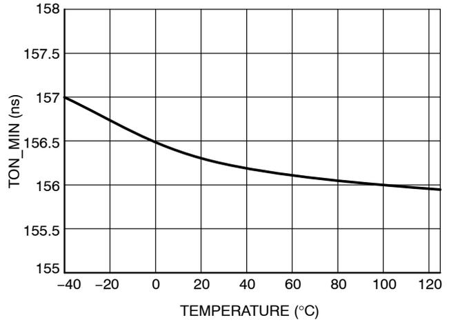
**Figure 17.  $T_{\text{ON\_MIN}}$  vs. T at  $V_{\text{HVBias}} = 48\text{ V}$**
