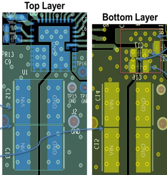
Place some vias on the VIN and PGND pads right under the device
