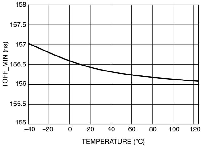
**Figure 18.  $T_{\text{OFF\_MIN}}$  vs. T at  $V_{\text{HVBias}} = 48\text{ V}$**
