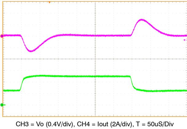
Figure 33. Load Step between 2.5 A and 5 A Load
