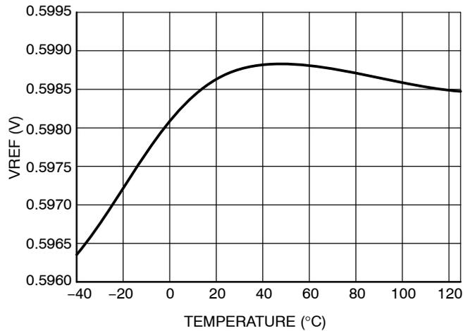
Figure 9.  $V_{\text{REF}}$  vs T at  $V_{\text{HVBIAS}} = 48\text{ V}$
