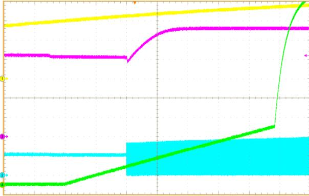
CH1 = Vin (10V/div), CH2 = SW (20V/div), CH3 = Vo (5V/div),
