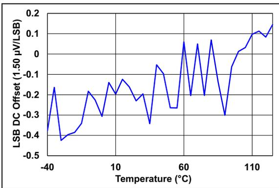
**FIGURE 2-19:** Input Offset for  $V_{SENSE}$  Measurements vs. Temperature.
