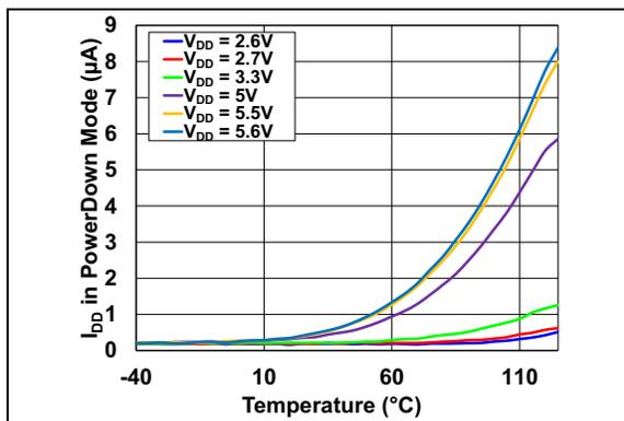
**FIGURE 2-25:** Power-Down Mode Current vs. Temperature and Supply.
