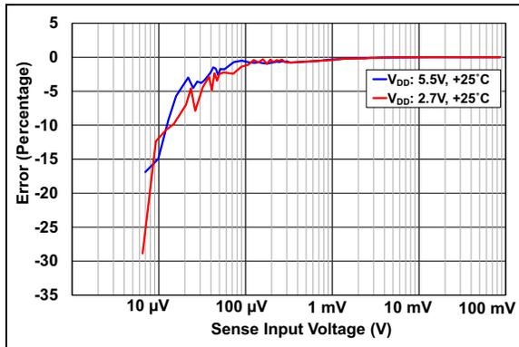
**FIGURE 2-1:**  $V_{SENSE}$  Error vs.  $V_{SENSE}$  Input Voltage.
