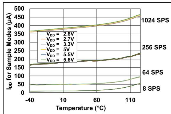
**FIGURE 2-23:**  $I_{DD}$  vs. Temperature, Supply and Sample Rate.
