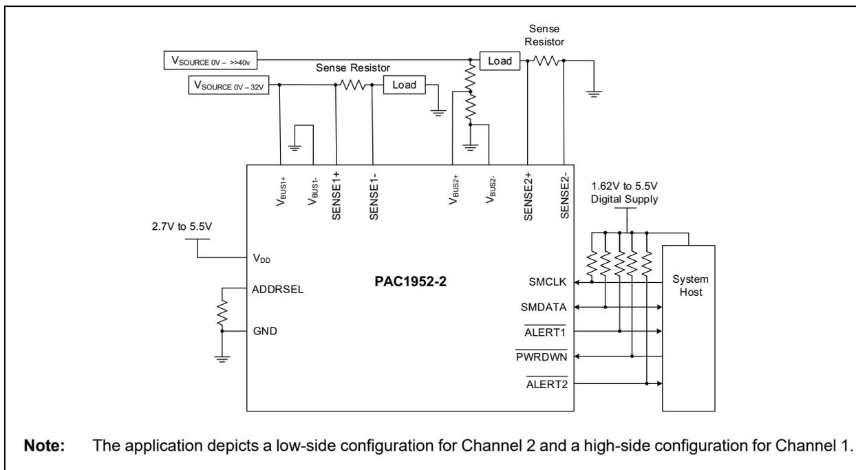
**Note:** The application depicts a low-side configuration for Channel 2 and a high-side configuration for Channel 1.
