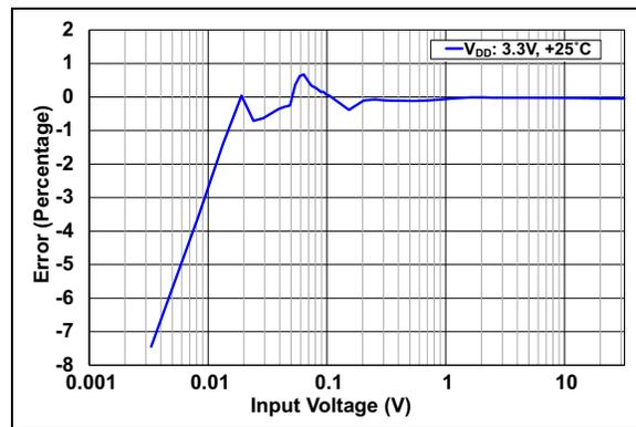
**FIGURE 2-11:**  $V_{BUS}$  Error vs.  $V_{BUS}$  Input Voltage.
