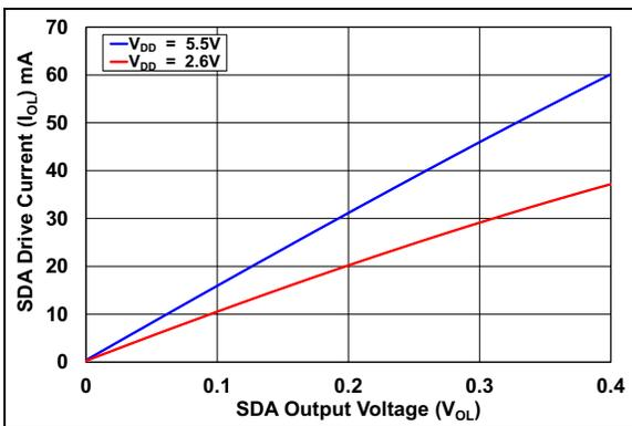
**FIGURE 2-20:** SDA Drive Current vs.  $V_{OL}$  at  $+25^\circ\text{C}$ .
