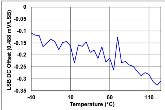
**FIGURE 2-18:** Input Offset for  $V_{BUS}$  Measurements vs. Temperature.
