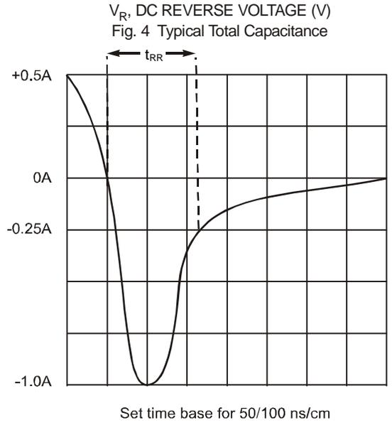
**Fig. 5 Reverse Recovery Time Characteristic and Test Circuit**
