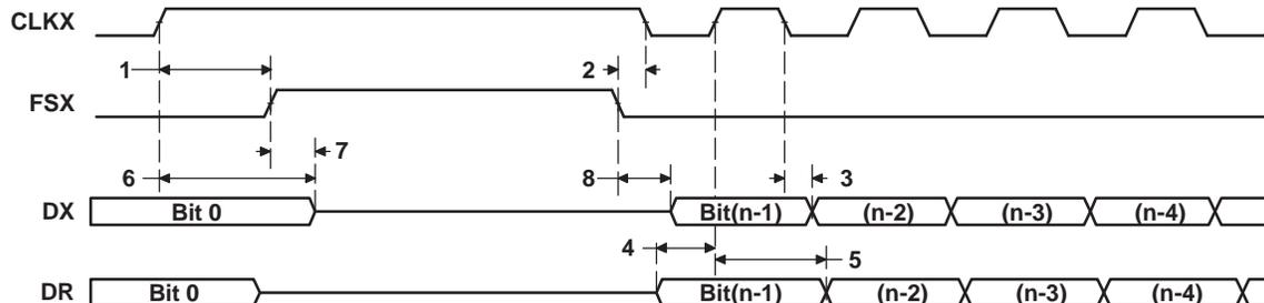
**Figure 5-55. McBSP Timing as SPI Master or Slave: CLKSTP = 10b, CLKXP = 1**
