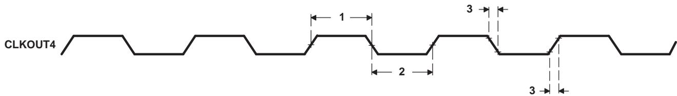
**Figure 5-12. CLKOUT4 Timing**
