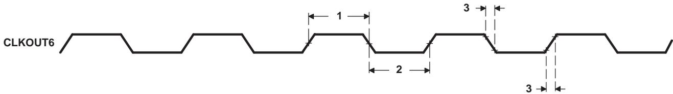
**Figure 5-13. CLKOUT6 Timing**
