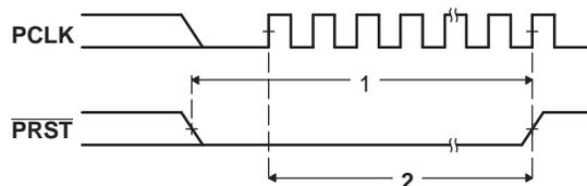
**Figure 5-47. PCI Reset ( $\overline{PRST}$ ) Timing**
