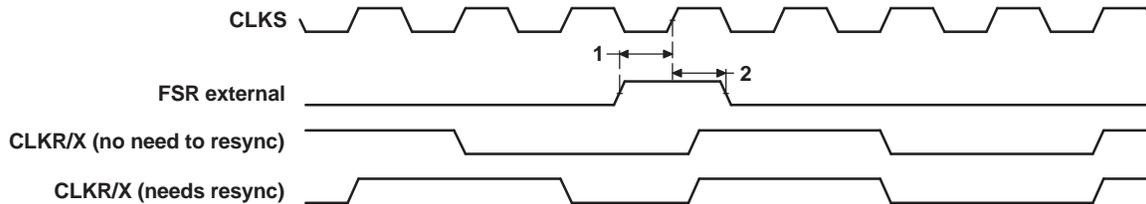
Figure 5-52. FSR Timing When GSYNC = 1
