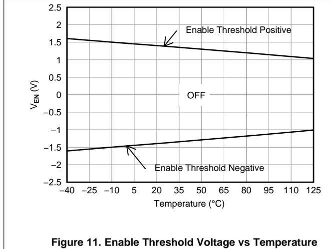
Figure 11. Enable Threshold Voltage vs Temperature
