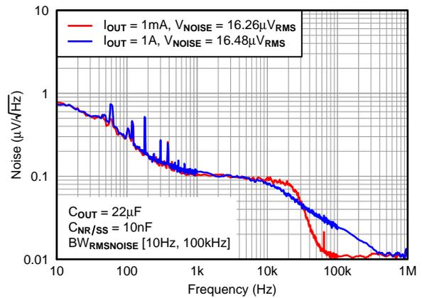
Figure 20. Output Spectral Noise Density vs Output Current
