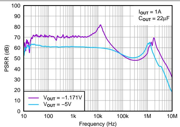
Figure 18. Power-Supply Rejection Ratio vs  $V_{OUT}$
