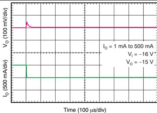
Figure 23. Load Transient
