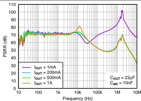
Figure 17. Power-Supply Rejection Ratio vs  $I_{OUT}$
