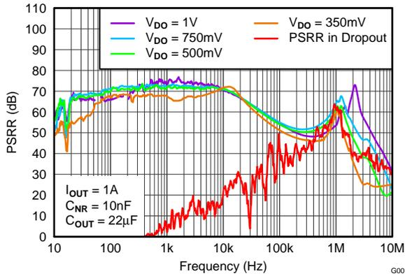
Figure 19. Power-Supply Rejection Ratio vs  $V_{DO}$
