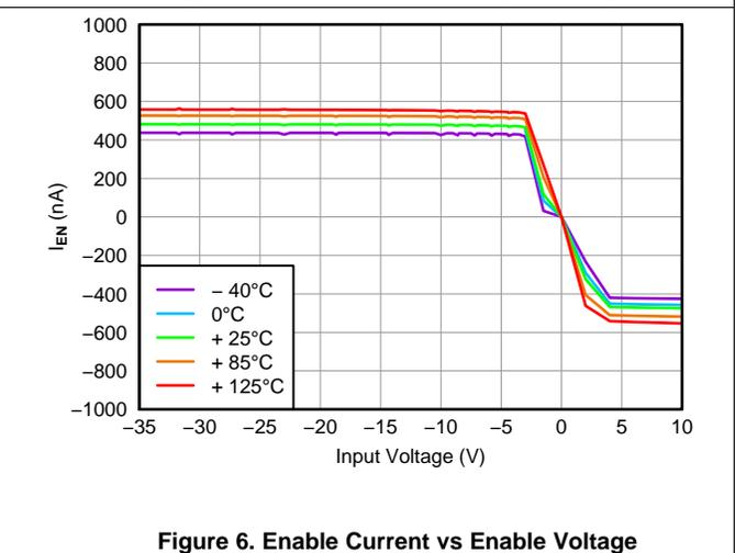
Figure 6. Enable Current vs Enable Voltage
