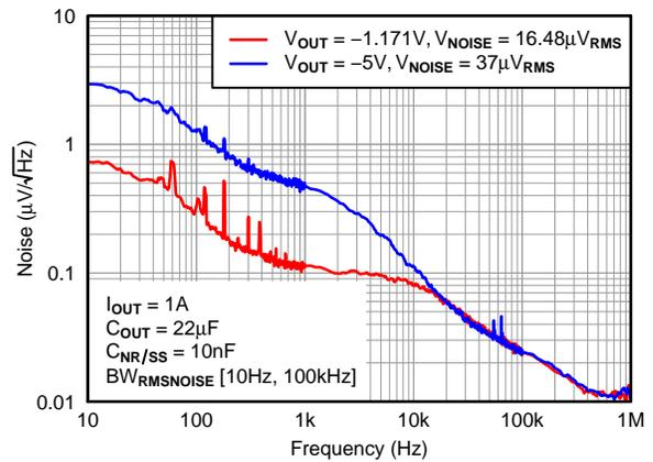
Figure 22. Output Spectral Noise Density vs  $V_{OUT(nom)}$
