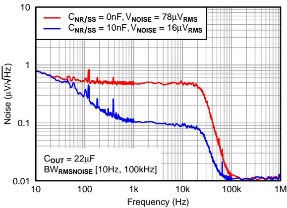
Figure 21. Output Spectral Noise Density vs  $C_{NR/SS}$
