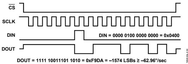
Figure 12. Example SPI Read, Second 16-Bit Sequence
