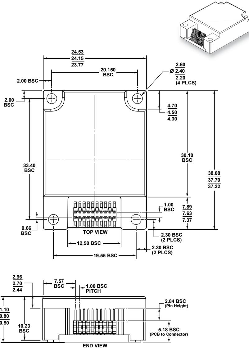
Figure 24. 20-Lead Module with Connector Interface [MODULE] (ML-20-3)
