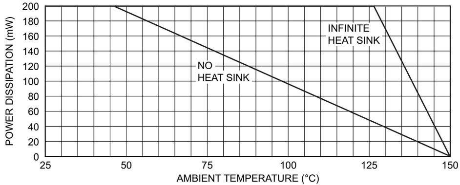
Typical Degradation Curve
