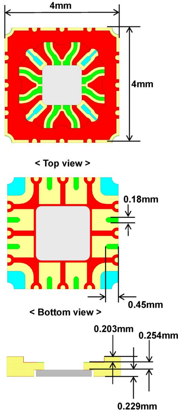
Fig. 4. CQFN 24-Pin Package Drawing (All Dimensions in mm)
