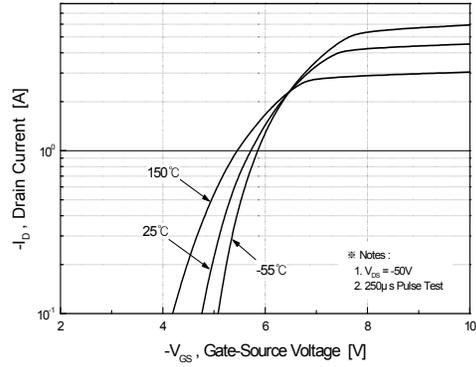
Figure 2. Transfer Characteristics
