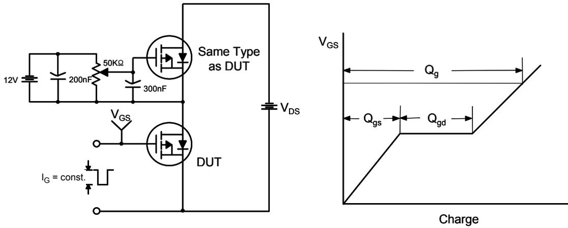
Figure 12. Gate Charge Test Circuit & Waveform
