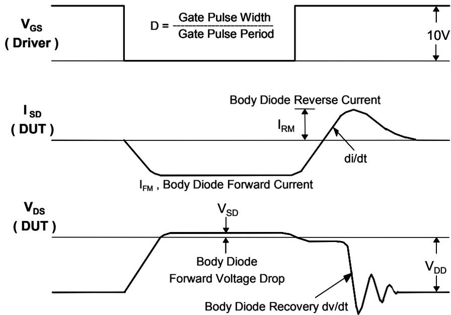
Figure 15. Peak Diode Recovery  $dv/dt$  Test Circuit & Waveforms
