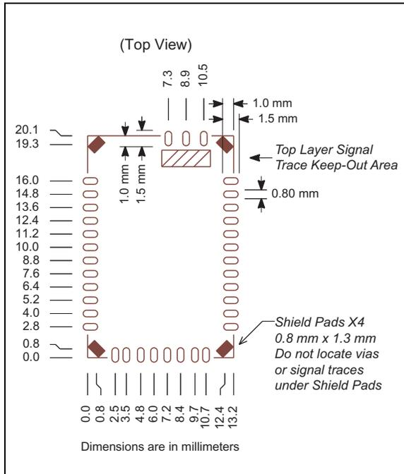
**FIGURE 2-4: RN41N MODULE MOUNTING DETAILS**
