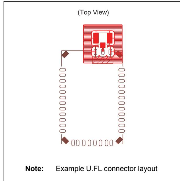
**FIGURE 2-3: RN41 MODULE MOUNTING DETAILS**
