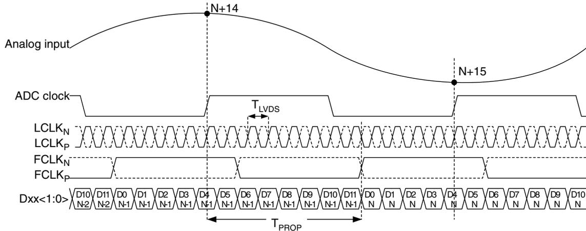
Figure 6. LVDS timing 12 bit output, SDR mode
