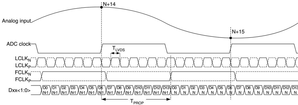
Figure 5. LVDS timing 14 bit output, DDR mode
