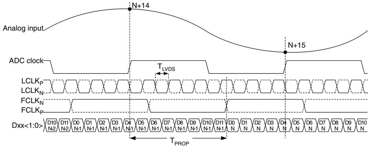
Figure 4. LVDS timing 12 bit output, DDR mode
