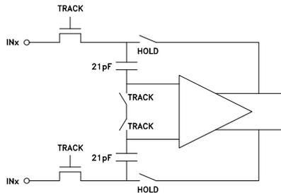
Figure 11. Input configuration
