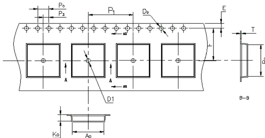
Figure 11 details the orientation of the CYBLE-014008-00 in the tape as well as the direction for unreeling.
