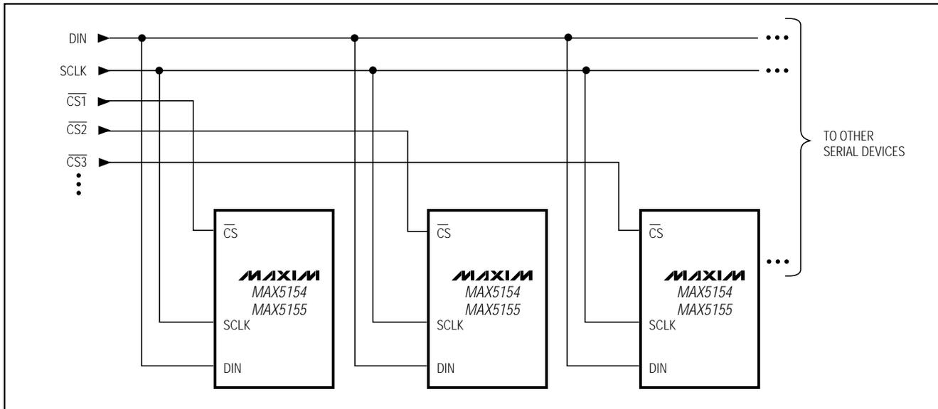
Figure 8. Multiple MAX5154/MAX5155s Sharing a Common DIN Line
