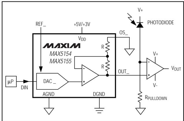
Figure 13. Digital Calibration
