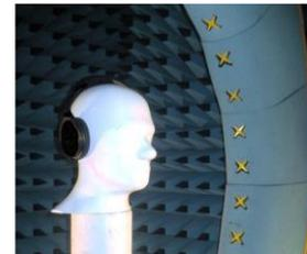
Anechoic chambers and full equipped in-house lab
