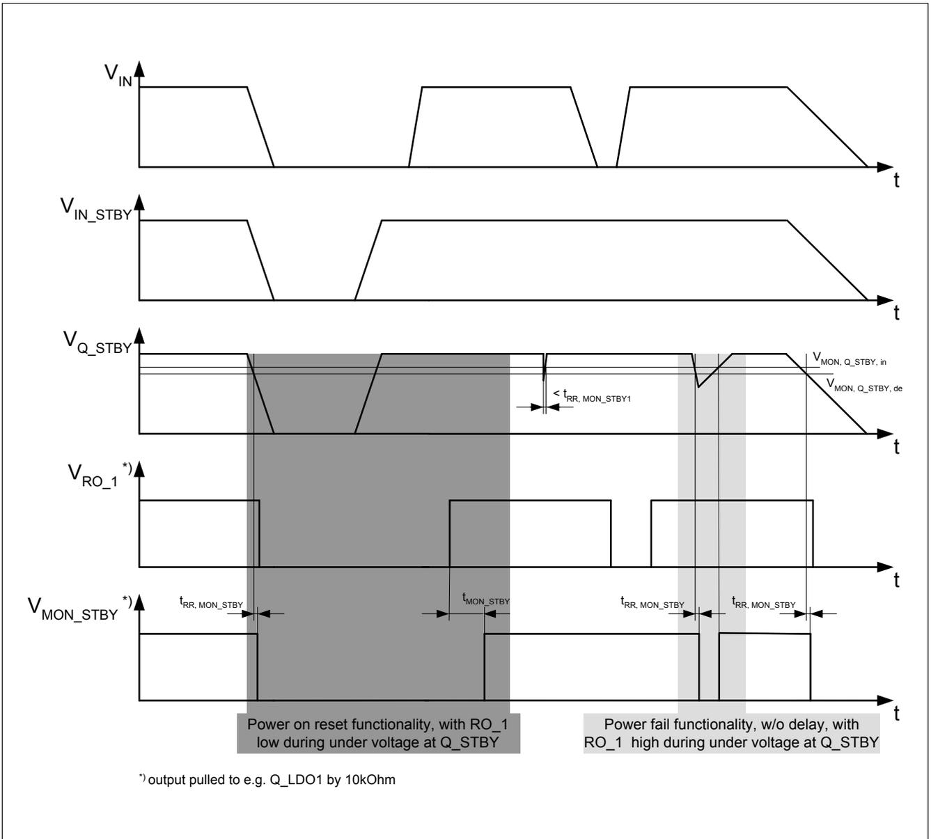
**Figure 7 Stand by Monitor Timing Diagram**
