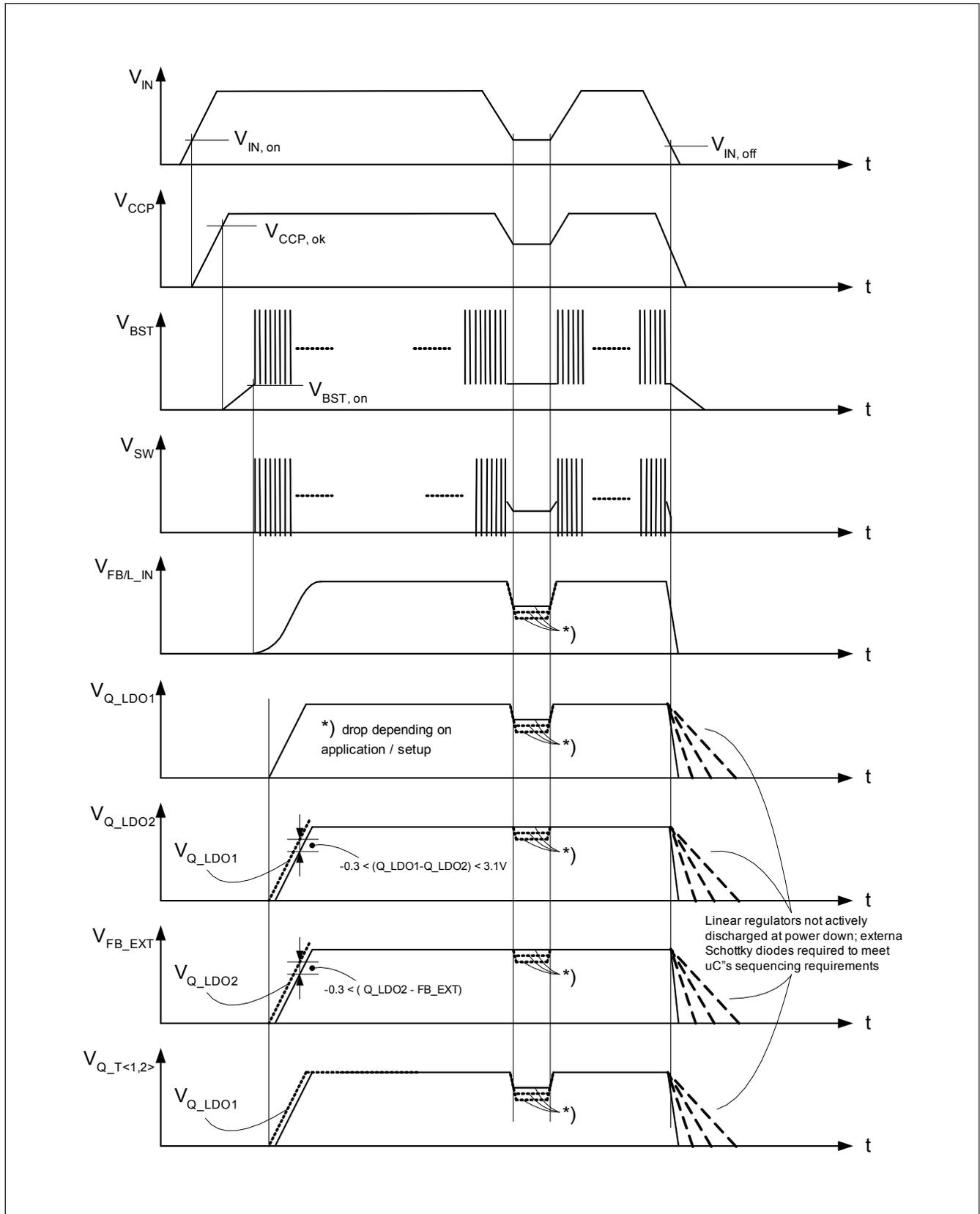
**Figure 4 Power Sequencing of the TLE7368**
