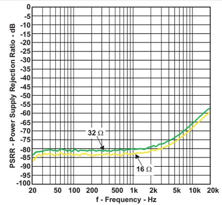
**Figure 6. Supply Rejection Ratio vs Frequency**
