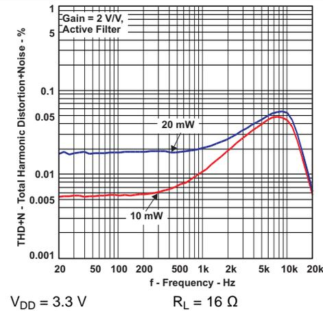
**Figure 4. Total Harmonic Distortion and Noise vs Frequency**
