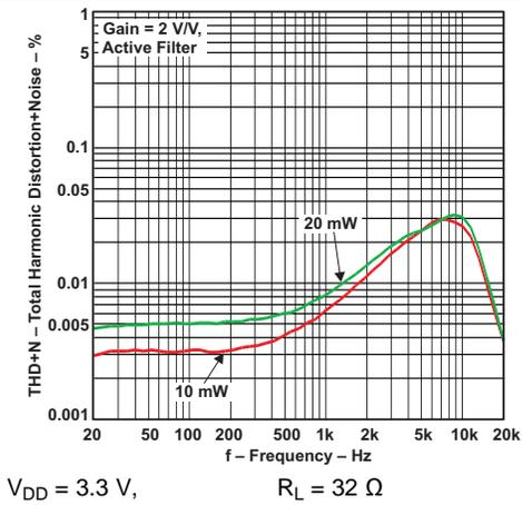
**Figure 3. Total Harmonic Distortion and Noise vs Frequency**
