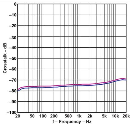
**Figure 5. Crosstalk vs Frequency**
