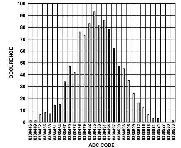
Figure 10. Histogram (Analog Input Buffers Disabled, V<sub>REF</sub> = 5 V, Output Data Rate = 31.25 kSPS)
