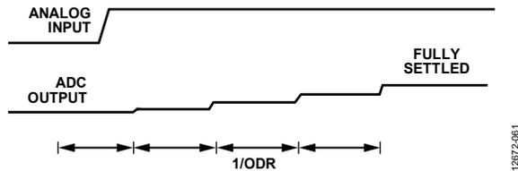
Figure 60. Step Input Without Single Cycle Settling
