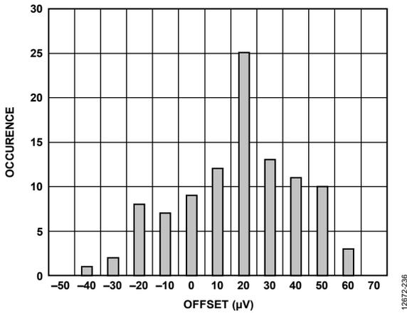
Figure 30. Offset Error Distribution Histogram (Internal Short, 100 Units)
