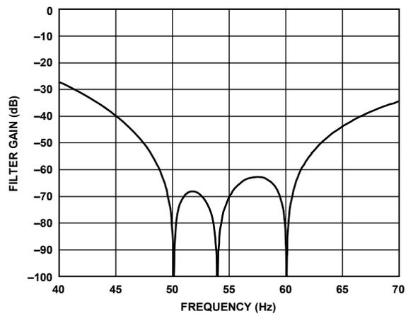
Figure 66. 25 SPS ODR, 40 ms Settling Time (40 – 70 Hz)
