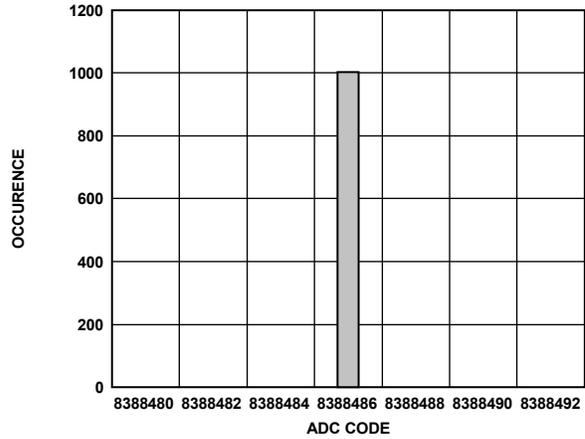
Figure 8. Histogram (Analog Input Buffers Disabled, V<sub>REF</sub> = 5 V, Output Data Rate = 1.25 SPS)
