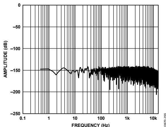
Figure 53. Shorted Input FFT (Analog Input Buffers Enabled)
