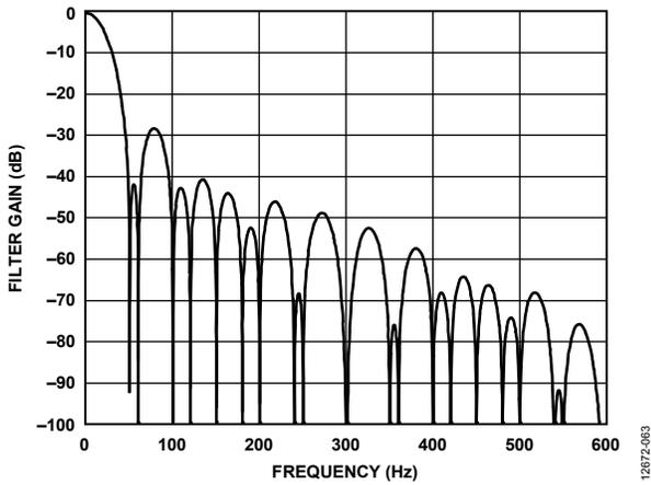
Figure 62. 27.27 SPS ODR, 36.67 ms Settling Time
