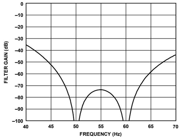
Figure 67. 20 SPS ODR, 50 ms Settling Time (40 – 70 Hz)
