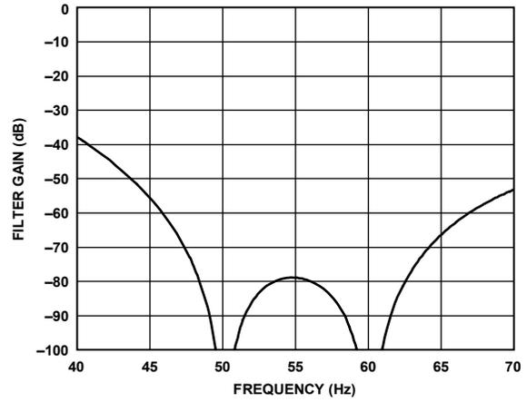
Figure 69. 16.667 SPS ODR, 60 ms Settling Time (40 – 70 Hz)
