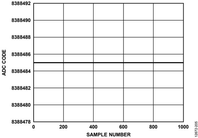
Figure 5. Noise (Analog Input Buffers Disabled, V<sub>REF</sub> = 5 V, Output Data Rate = 1.25 SPS)
