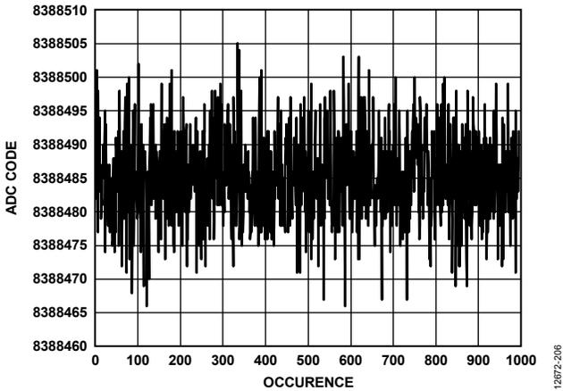
Figure 6. Noise (Analog Input Buffers Disabled, V<sub>REF</sub> = 5 V, Output Data Rate = 2.6 kSPS)
