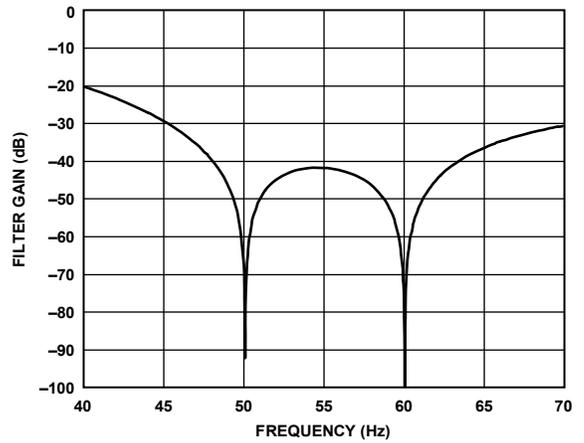
Figure 65. 27.27 SPS ODR, 36.67 ms Settling Time (40 – 70 Hz)
