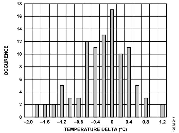
Figure 38. Temperature Sensor Distribution Histogram (Uncalibrated, 100 Units)
