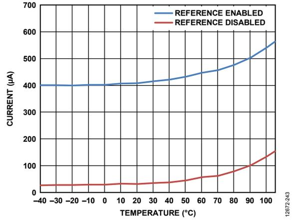
Figure 37. Current Consumption vs. Temperature (Standby Mode)
