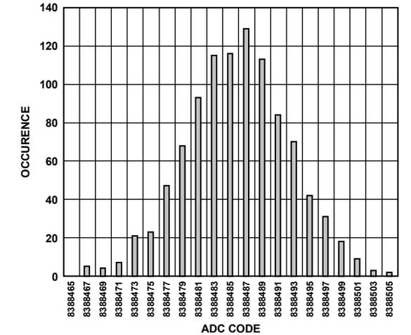
Figure 9. Histogram (Analog Input Buffers Disabled, V<sub>REF</sub> = 5 V, Output Data Rate = 2.6 kSPS)
