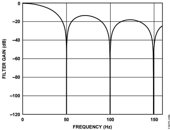
Figure 58. Sinc5 + Sinc1 Filter Response at 50 SPS ODR
