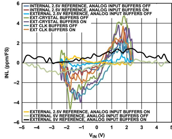
Figure 21. Integral Nonlinearity (INL) vs.  $V_{IN}$  (Differential Input)
