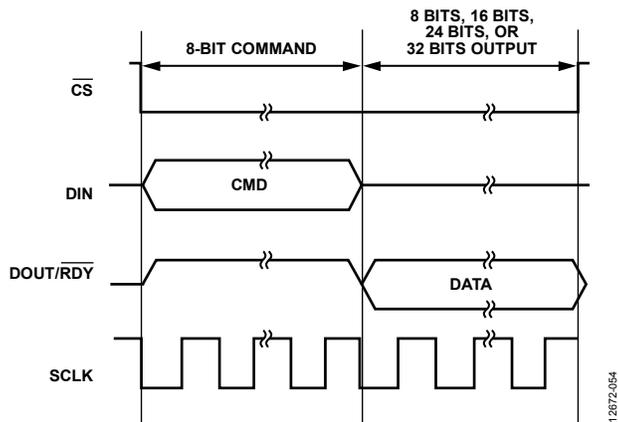
Figure 47. Reading from a Register
