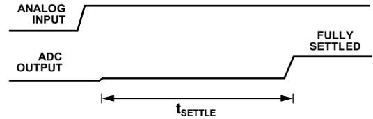
Figure 61. Step Input with Single Cycle Settling
