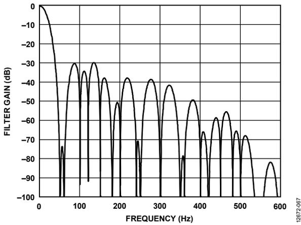
Figure 64. 20 SPS ODR, 50 ms Settling Time
