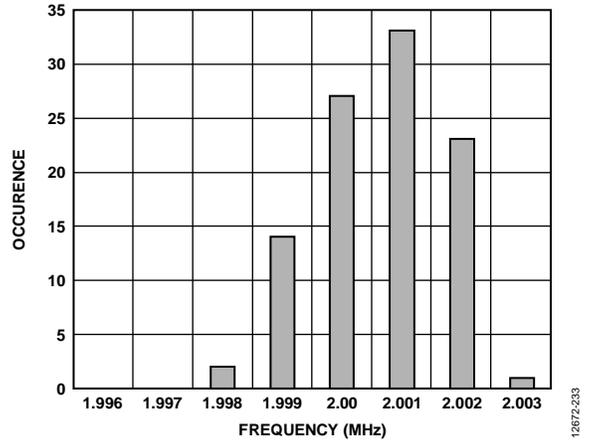
Figure 27. Internal Oscillator Frequency Distribution Histogram (100 Units)
