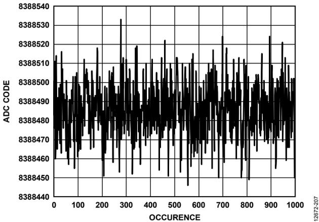
Figure 7. Noise (Analog Input Buffers Disabled, V<sub>REF</sub> = 5 V, Output Data Rate = 31.25 kSPS)
