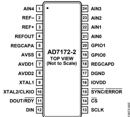
Figure 4. Pin Configuration
