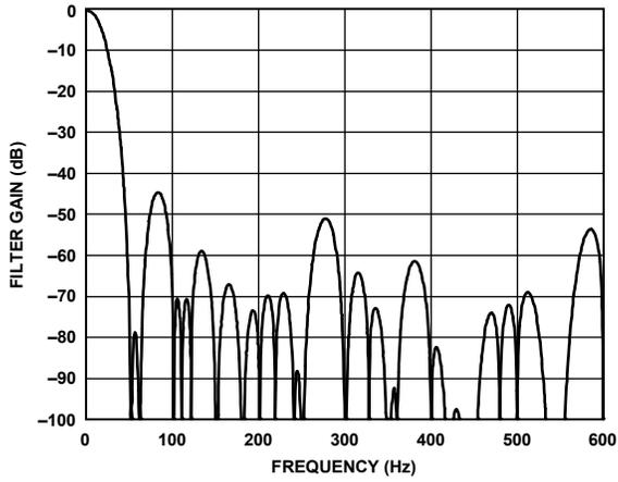
Figure 68. 16.667 SPS ODR, 60 ms Settling Time
