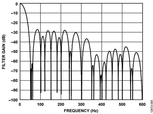
Figure 63. 25 SPS ODR, 40 ms Settling Time
