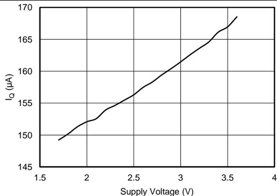
**Figure 10. Quiescent Current vs Supply Voltage (At Default Conversion Rate of 16 Conversions per Second)**
