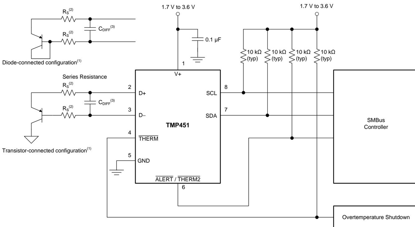
(1) Diode-connected configuration provides better settling time. Transistor-connected configuration provides better series resistance cancellation.
