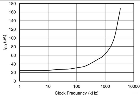
**Figure 9. Shutdown Quiescent Current vs SCL Clock Frequency**
