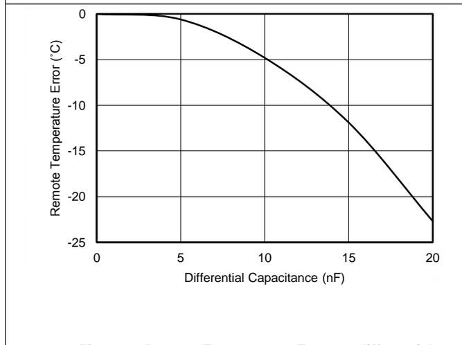
Figure 6. Remote Temperature Error vs differential Capacitance
