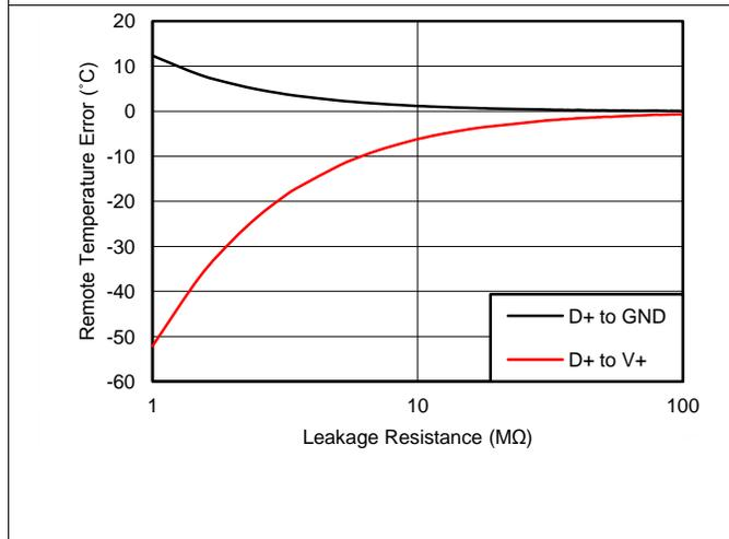
Figure 4. Remote Temperature Error vs Leakage Resistance
