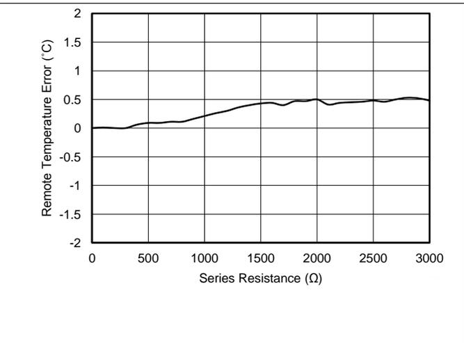
Figure 5. Remote Temperature Error vs Series Resistance
