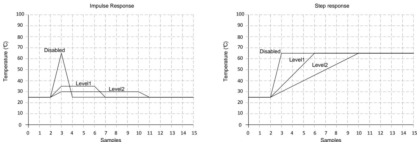
**Figure 12. Filter Response to Impulse and Step Inputs**
