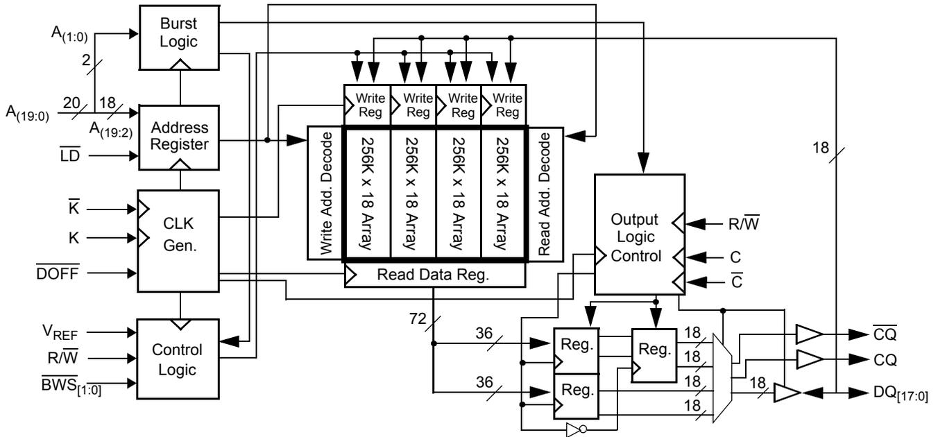
Logic Block Diagram – CY7C1321KV18
